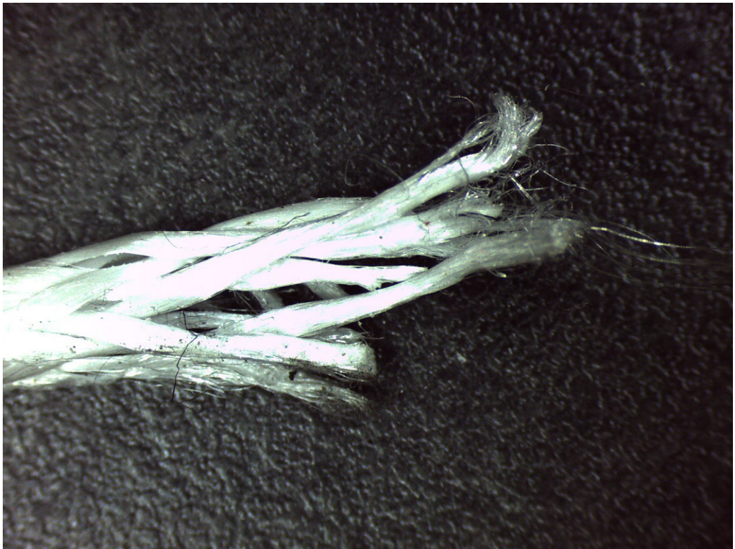
Figure 5: Cut and tear point of the connecting rope
