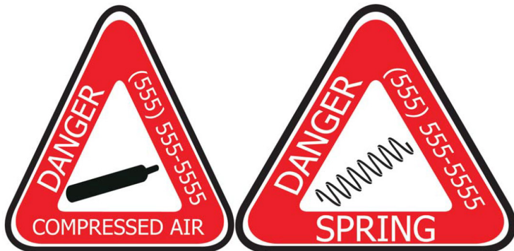
Figure 11: Sample of danger and warning labels for first responders (source: F3322)
