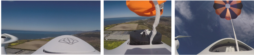
Figure 2: Image sequence of the parachute ejection during a test of the autonomous flight termination system (FTS). There are no danger and warning labels for first responders on the drone (source: Matternet).
