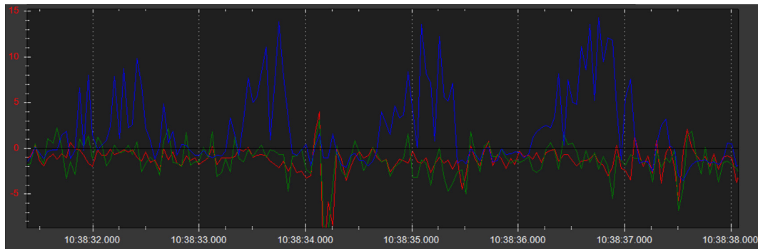
Figure 10: Time section (10:38:31 to 10:38:38) of the course of the deviations from the values of the acceleration sensors using IMU1 (red), IMU2 (green) and IMU3 (blue). From about 10:38:32, a clear oscillation (blue line) with a frequency of about 2/3 Hz can be seen.
