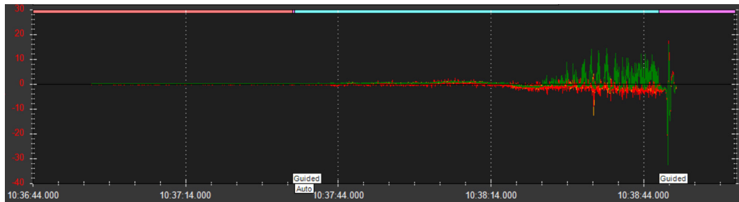
Figure 8: Time course of the deviations from the dimensionless values of the accelerometers using IMU1 (orange), IMU2 (red) and IMU3 (green).
