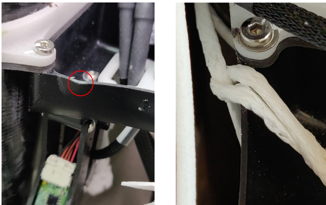
Figure 6: Clearly visible deformation of the sharp-edged attachment point (red circle) on the SUI-9903 drone involved in the accident (left) as well as the intact attachment of the connecting rope of an identical drone (right).
