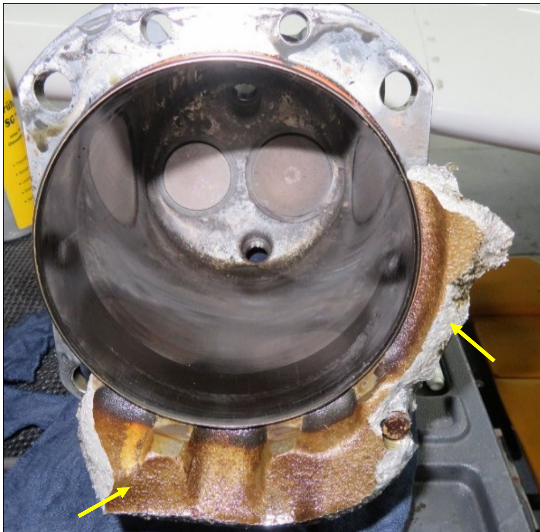
Figure 2: Cylinder #1 with cracked engine case (yellow arrows).
