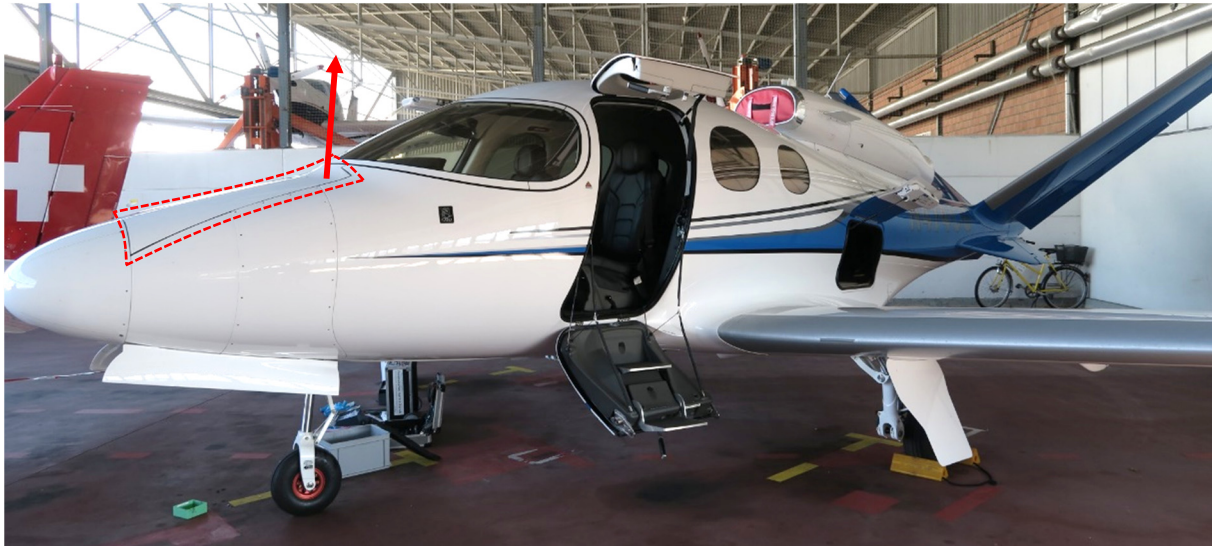
Figure 4: CAPS deployment opening (red dashed line) on the upper part of the front fuselage and direction of deployment of the rocket for the rescue parachute (red arrow).
