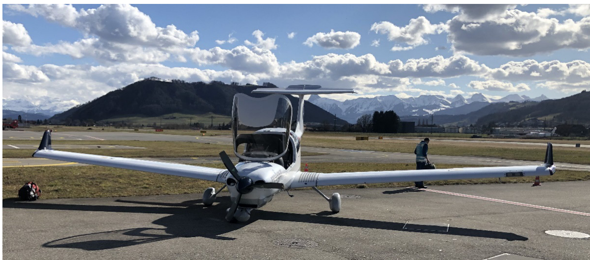
Figure 1: HB-SGD with collapsed nose gear on the apron of Bern-Belp Airport, view direction south.
