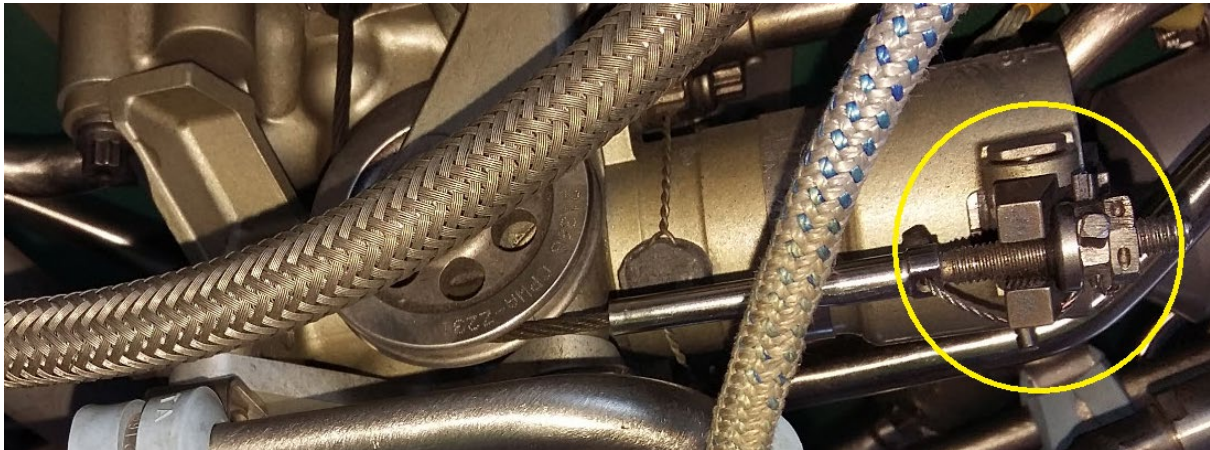
Figure 2: The emergency fuel shut-off valve with its actuating lever and its adjustable connection (yellow circle) to the Bowden cable via a pulley.
