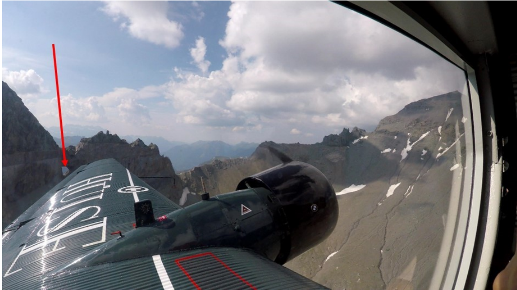
Figure 3: Still image from a video at point F10, recorded from the cabin of HB-HOT looking towards the Martinsloch (red arrow). The pitch attitude was 11.0 degrees, the left bank attitude 4.8 degrees and the altitude 2,749 m AMSL. The difference between the flight path angle and the pitch angle was 20.6 degrees.
