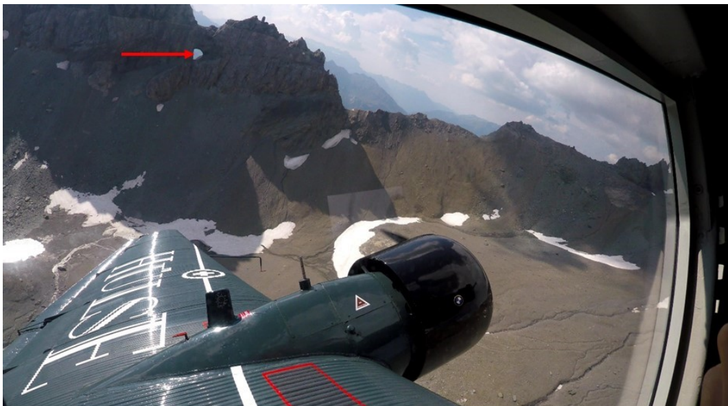
Figure 4: Still image from a video at point F13, recorded from the cabin of HB-HOT looking towards the Martinsloch (red arrow), 4.3 seconds after the image shown in figure 3 was taken. The pitch attitude was 12.1 degrees, the left bank attitude 32.7 degrees and the altitude 2,724 m AMSL.
