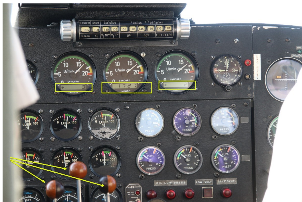
Figure 4: Tachometers with digital displays, marked by yellow rectangles. The yellow arrows point to the three throttle levers that must be operated to set the respective rpm.
