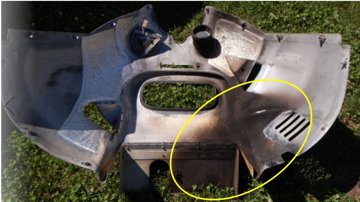
Figure 1: Front engine cowling after removal with evident oily soot deposit on the lower right part, in the region of the hot section of the turbocharger (yellow ellipse)
