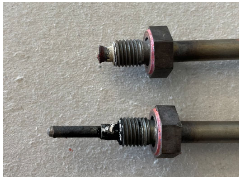
Figure 3: Exhaust gas temperature probe. The missing part of the damaged probe (above) is highlighted by comparing the damaged probe to an undamaged probe (below).
