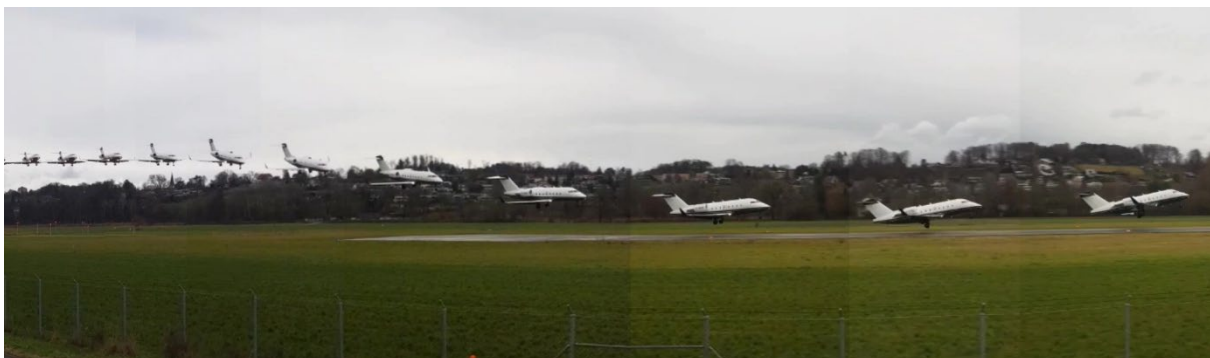
Figure 1: Video recording by a passerby of the G-XONE’s go-around over the area of Runway 14 located in front of the threshold (eleven individual frames taken one second apart, combined into a single image).
