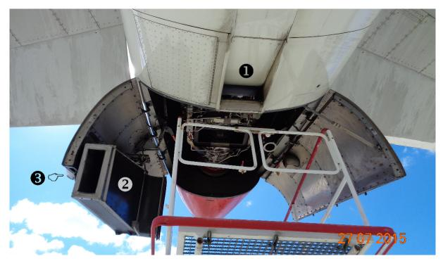
**Illustration 1:** View of the open APU bay in the aircraft's tail cone. The air required for the operation of the APU is sucked in through the air inlet (1) and reaches the APU via the air inlet duct (2) attached to the hatch. When the APU bay is closed, the top of the air inlet duct acts as a drip tray, which is emptied to the outside via the drain mast (3); the drain mast is located directly behind the air inlet.
