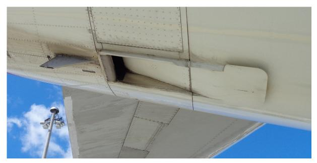
**Illustration 2:** View of the open APU inlet duct on the underside of the aircraft's tail cone. The drain mast can be seen to the left of it.
