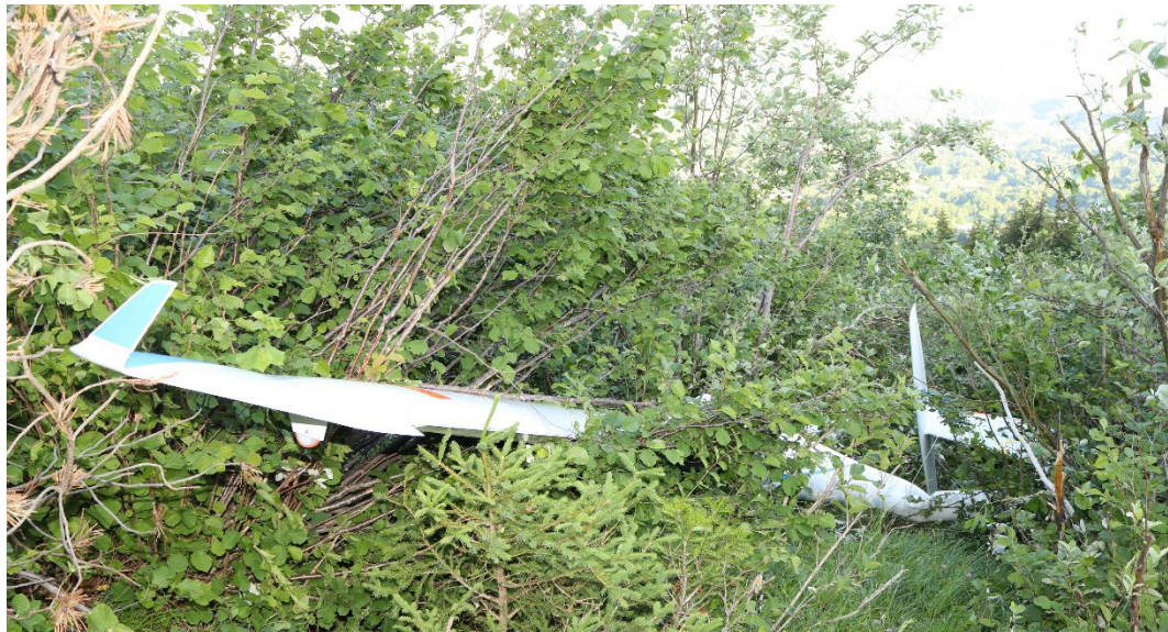
Figure 2: Wreckage of the D-MANS as it appeared to the rescue forces arriving at the accident site. It cannot be identified that there was a risk of electric shock and that no ballistic parachute system was installed (photo by the Valais Cantonal Police).
