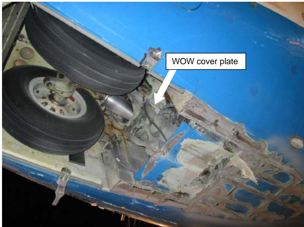
Figure 2: The nose gear WOW cover plate squeezed between the lower and the upper drag strut of the nose landing gear. The picture was taken on the accident site.
