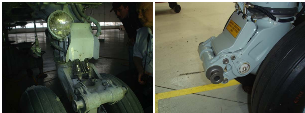
Figure 1: Left side: WOW cover plate found after lowering the nose landing gear. Right side: Normal WOW cover plate installation.
