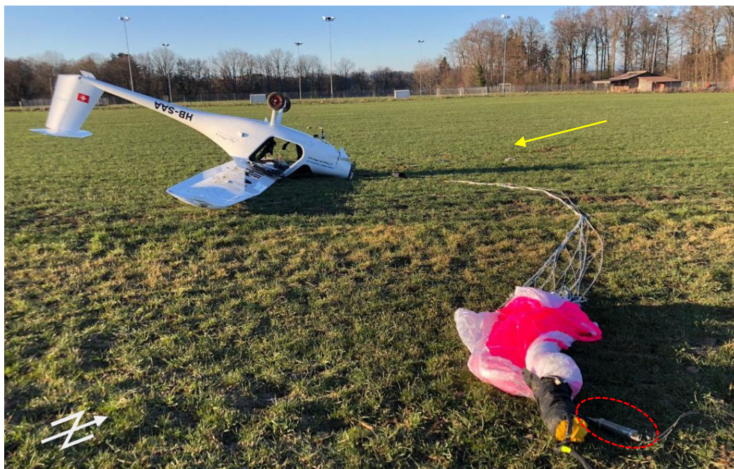
Figure 2: Final position of the aircraft (landing direction yellow arrow) with ejected, partially deployed rescue parachute and deployed rocket (red circle). The Corpataux-Magnedens (FR) sports ground is visible in the background.
