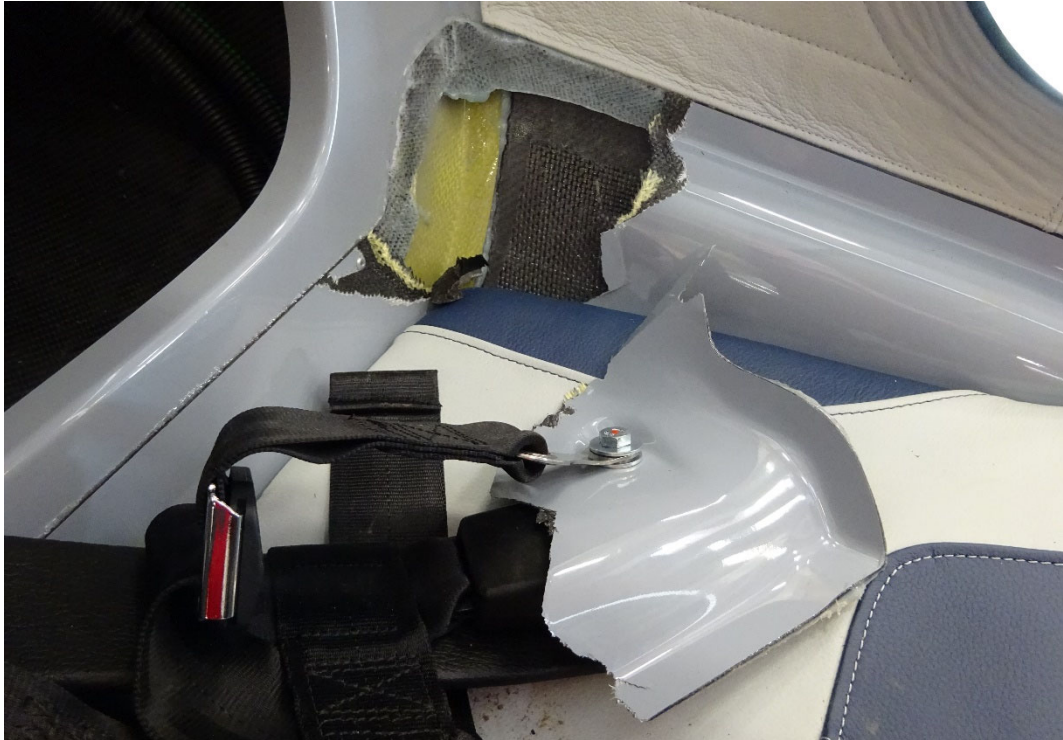
Figure 8: Torn off attachment point of the pilot's left lap belt.
