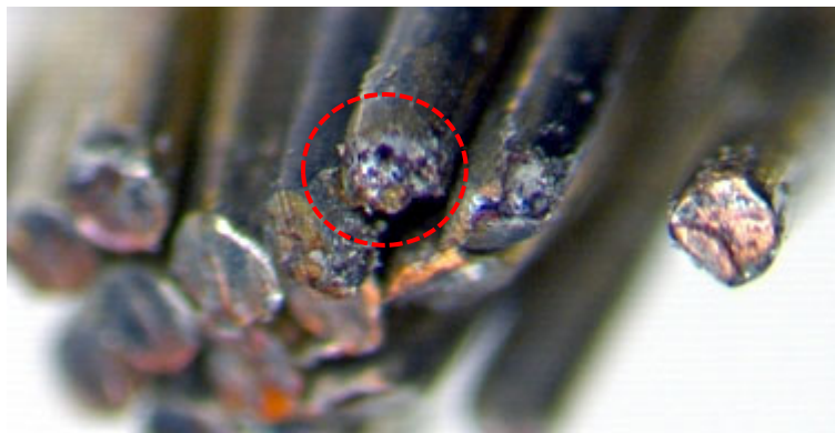
Figure 7: Close-up of the end of the red power supply cable. Traces of burning (electric arcs) can be seen on several copper wires (red circle).
