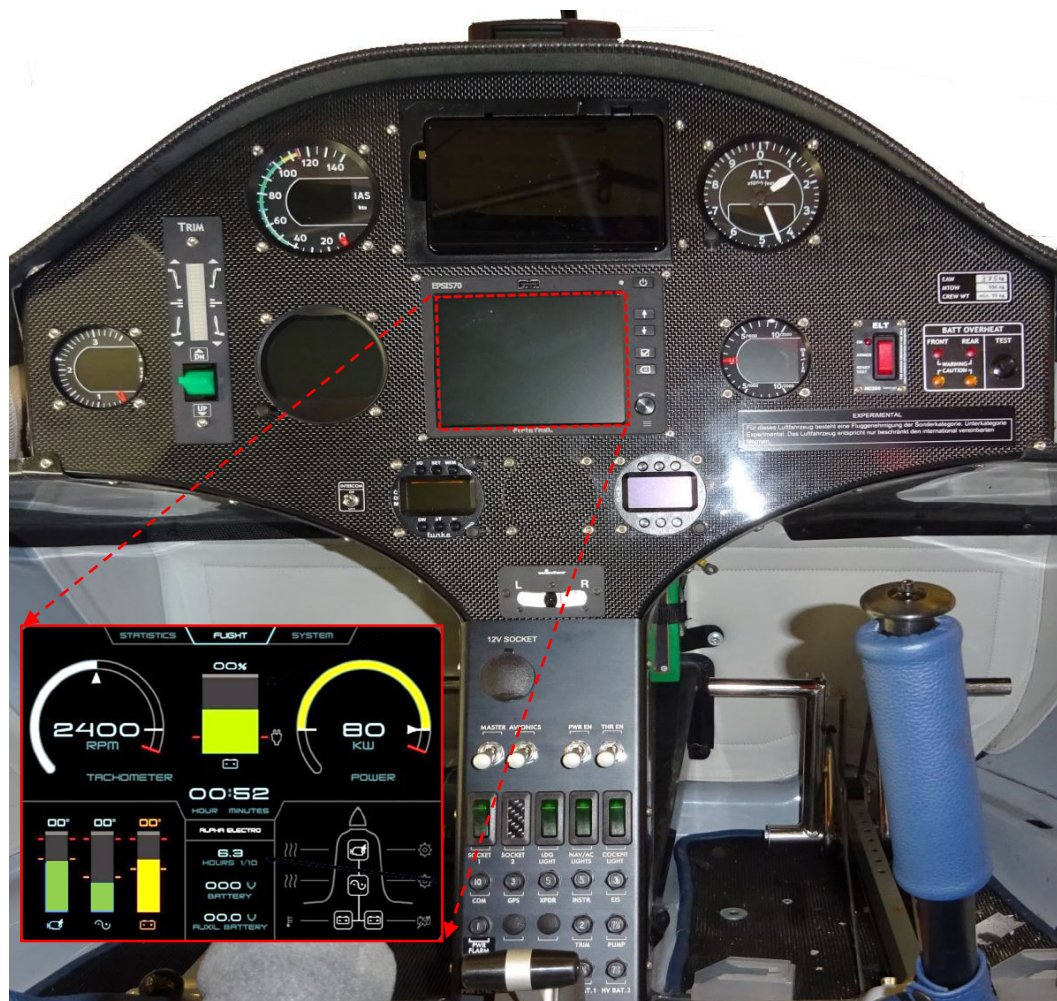
Figure 4: Instrument panel of HB-SAA with EPSI (circled with red dashes, source Pipistrel). The main page of the EPSI has been enlarged (values do not correlate).
