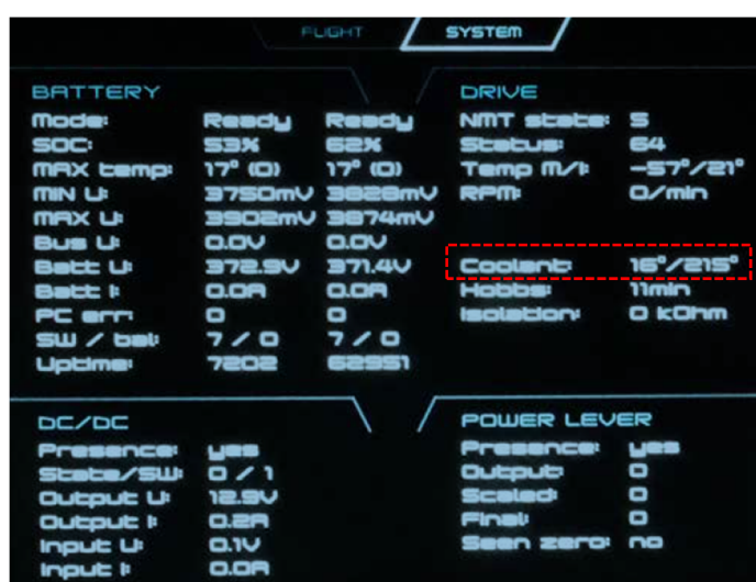
Figure 5: System page with various parameters of the propulsion unit, including the coolant temperatures (circled in red). Source: Pipistrel.
