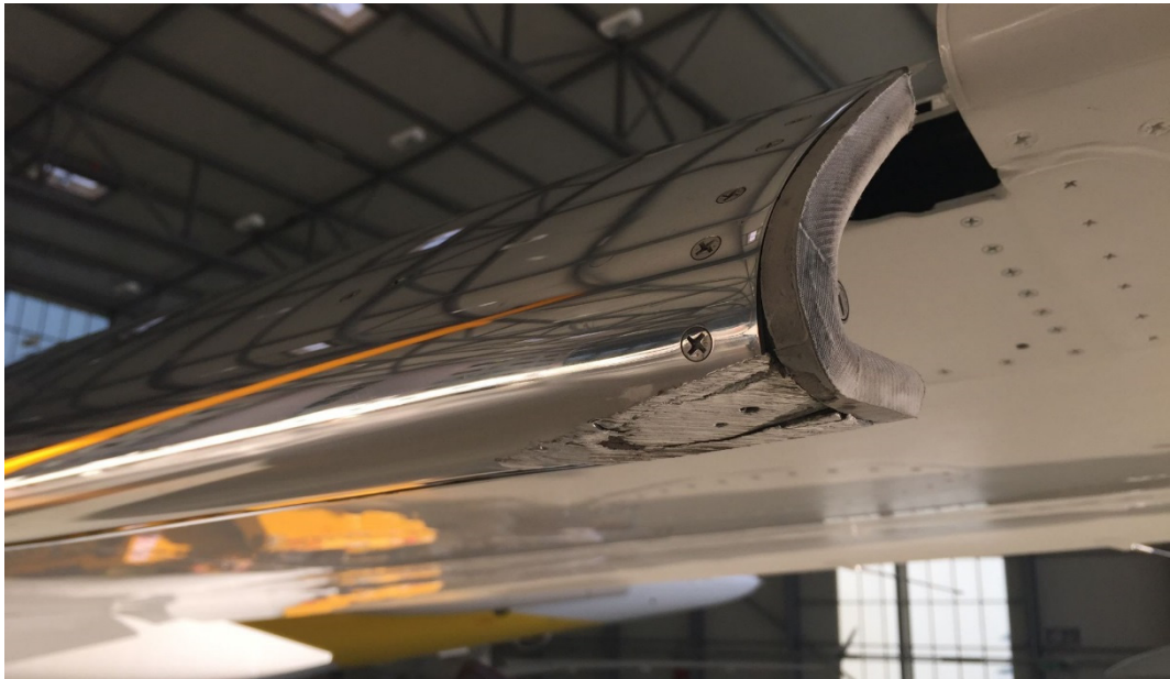
Illustration 2: Left outer leading-edge slat shown in its extended position with scratch and rubbing marks on the underside
