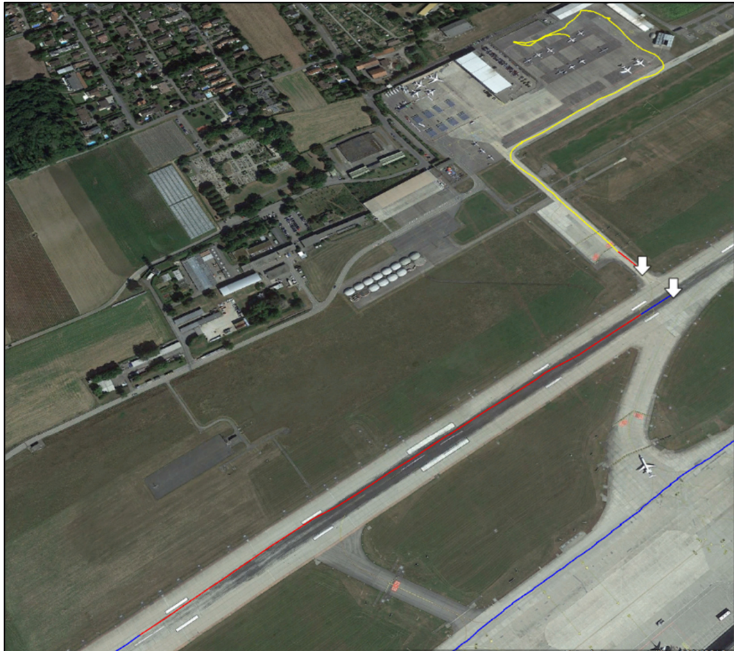
Figure 1: Paths of N990FV (yellow) and EIN68N (blue). The parts shown in red indicate when the “RIMCAS” aural warning was generated.
