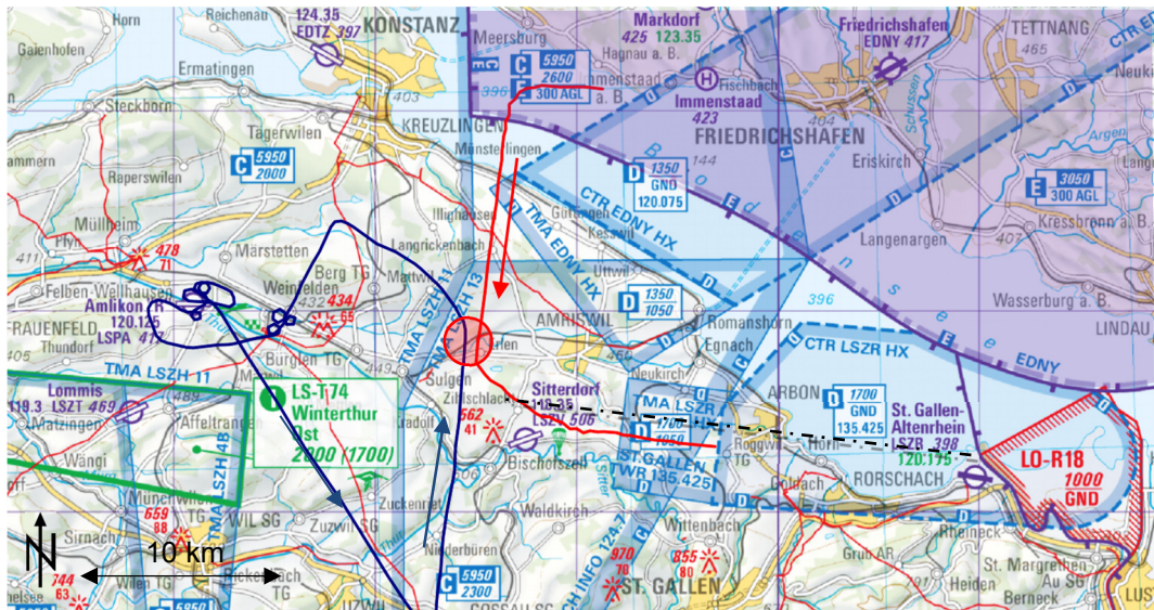
Illustration 1: Recordings of the flight paths of HB-3442 (blue) and CS-DLB (red), marked on the glider map of Switzerland. The final approach to ILS 10 St. Gallen-Altenrhein is marked as a dashed black line. The point of closest proximity is marked with a red circle. The Transponder Mandatory Zone (TMZ) around Friedrichshafen Airport is highlighted in purple. Source of base map: Swiss Federal Office of Topography.
