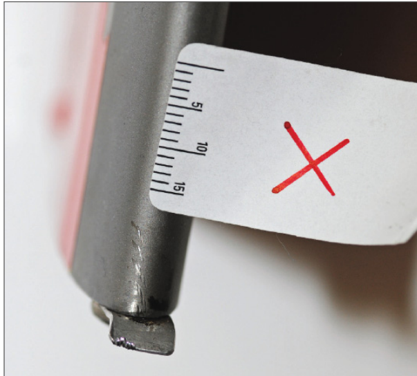
Illustration 9: The indentation on the strike indicator and contact mark on the tail rotor blade's leading edge (no. 1).
