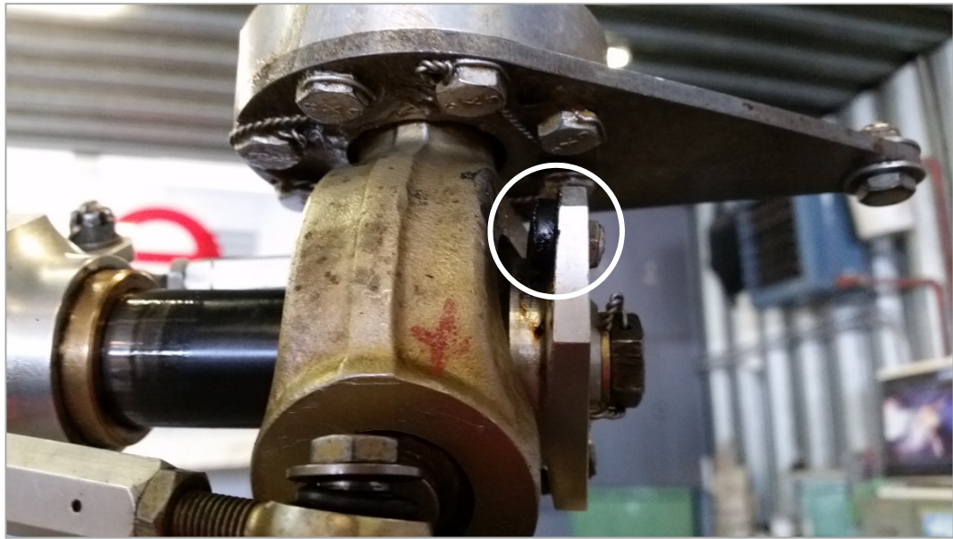
Illustration 5: The tail rotor driveshaft of HB-XLS with hub and static stop showing a defective rubber teeter stop bumper (circled in white). This photograph was taken on the day of the accident.
