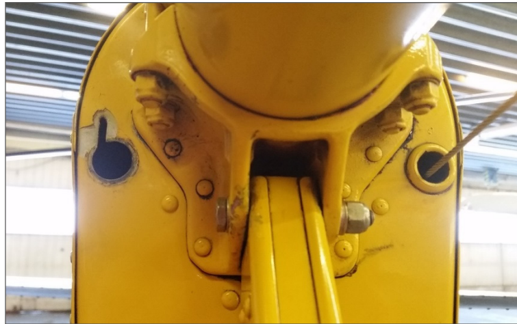
Illustration 11: The tail boom's rearmost bulkhead with the incision in the left fairlead.
