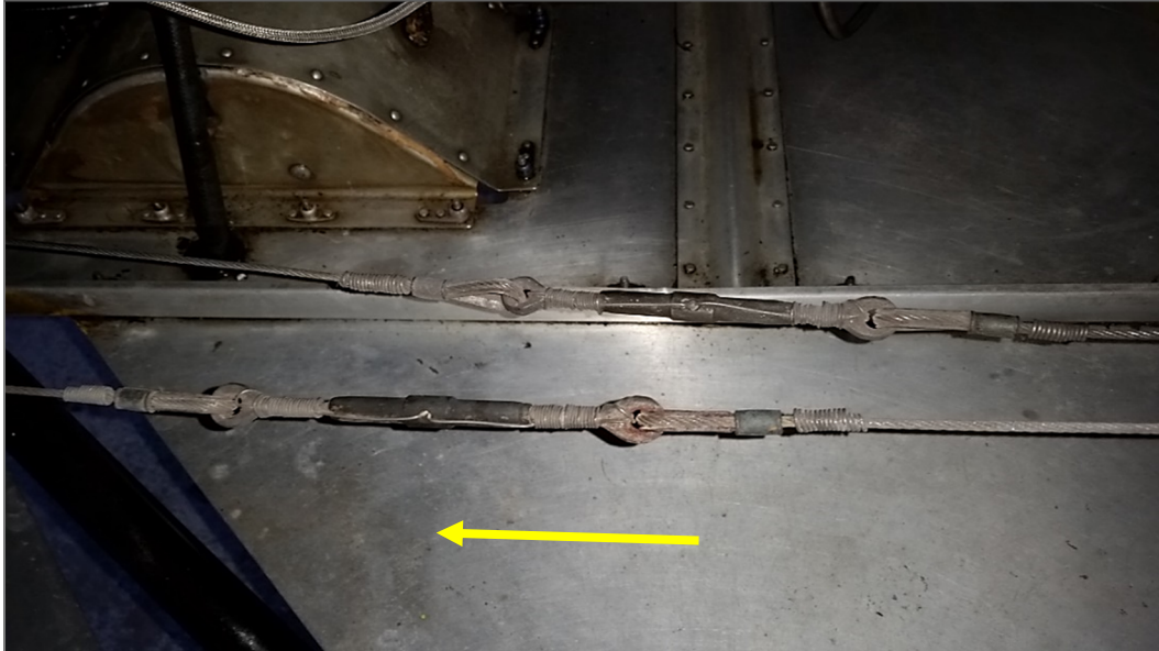
Illustration 4: The turnbuckles of the right and left tail rotor control cables with safety wire to prevent undesired loosening. In HB-XLS, they are located near the engine. The yellow arrow indicates the direction of flight.
