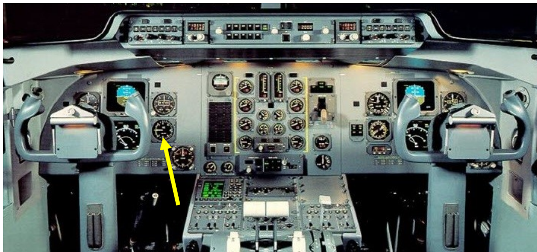
Figure 2: Flight deck of a Fokker 50. The yellow arrow shows the installation location of the commander's variometer. The copilot's instrument is concealed by the right control column.
