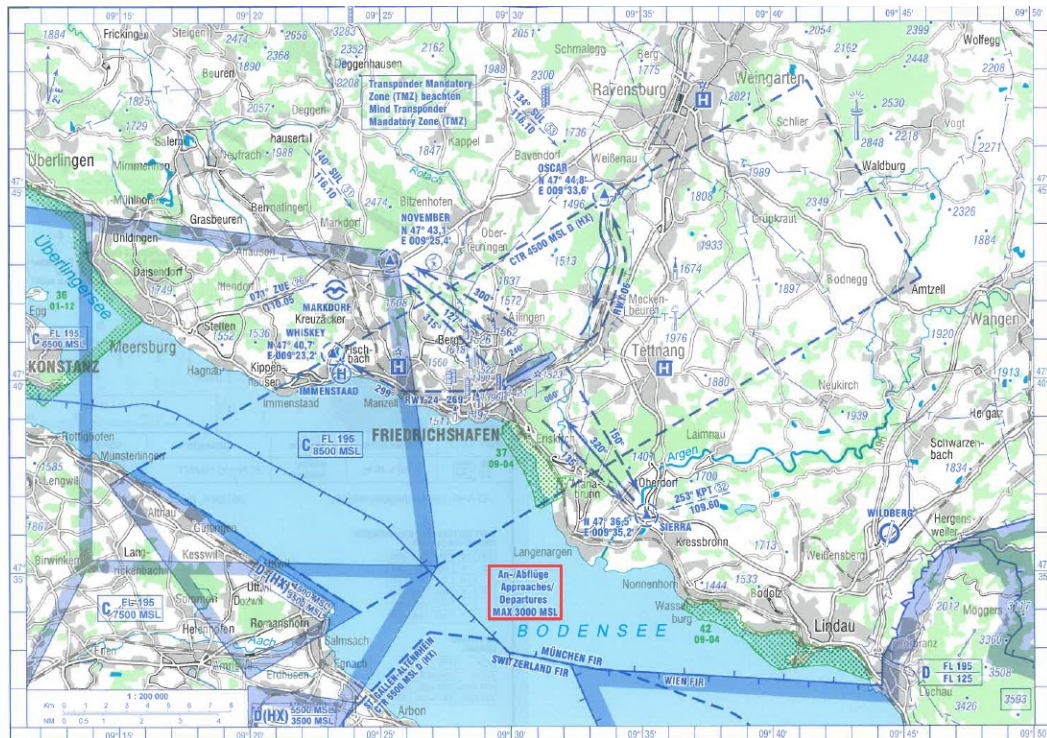
Figure 6: Visual approach chart for the airport of Friedrichshafen as per the aeronautical information publication (AIP) for Germany with a maximum flight altitude of 3000 ft AMSL for arrivals and departures (red frame)
