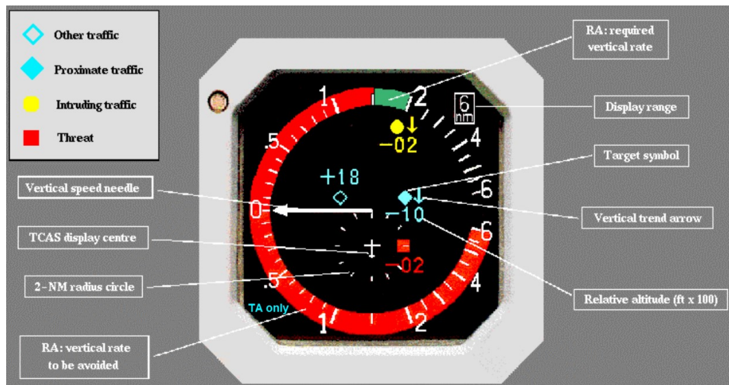
Figure 3: Illustration of the working principle of an integrated vertical speed indicator with a display function for the traffic alert and collision avoidance system. The relative altitudes of the other aircraft equipped with a transponder transmitting altitude data are indicated in hundreds of feet. The „TA only“ (blue) message appears in the lower left corner of the instrument display if the TCAS is in the mode „traffic advisories (TA) only“.
