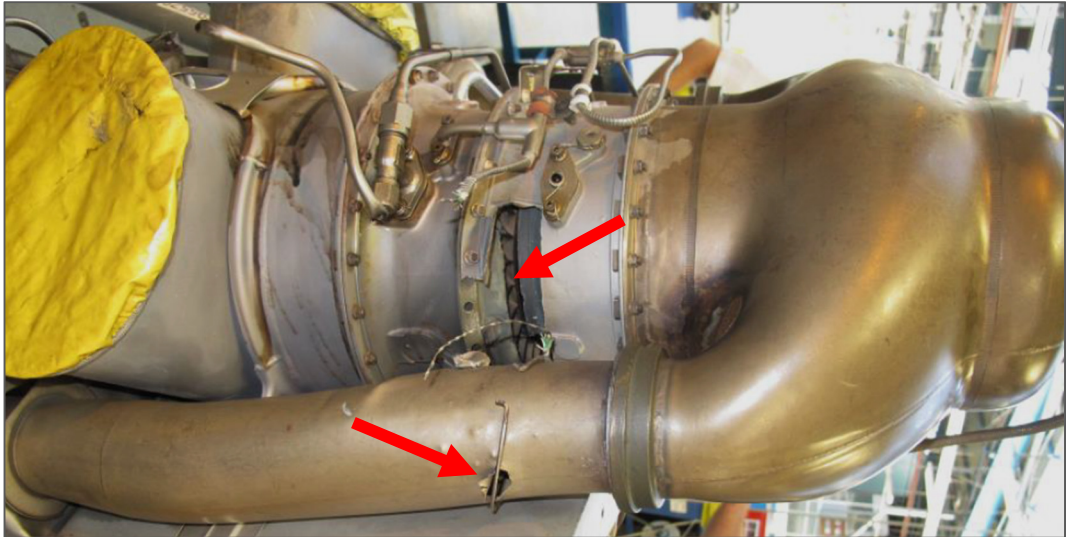
Illustration 6: Removed engine of HB-XSL with destroyed turbine module and damaged discharge tube (red arrows)
