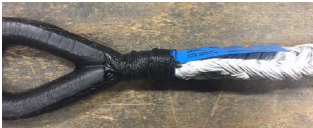
Figure 12: Example of an end of a longline with thimble and label. This longline also does not have a protective cover.
