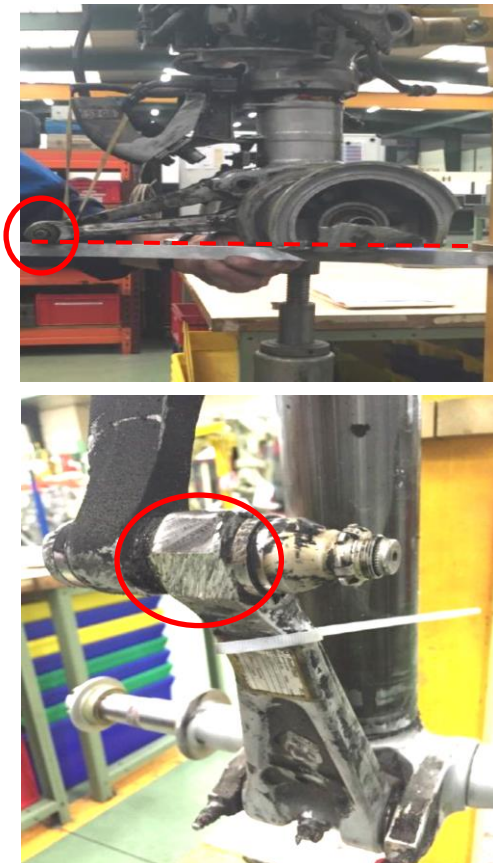
Figure 12: At the linkage between the upper and lower torque link both rod end bearings exhibited abrasion marks on the lower side.
