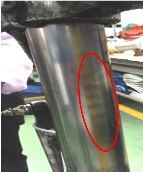
Figure 11: Markings on the sliding rod of the NLG assembly
