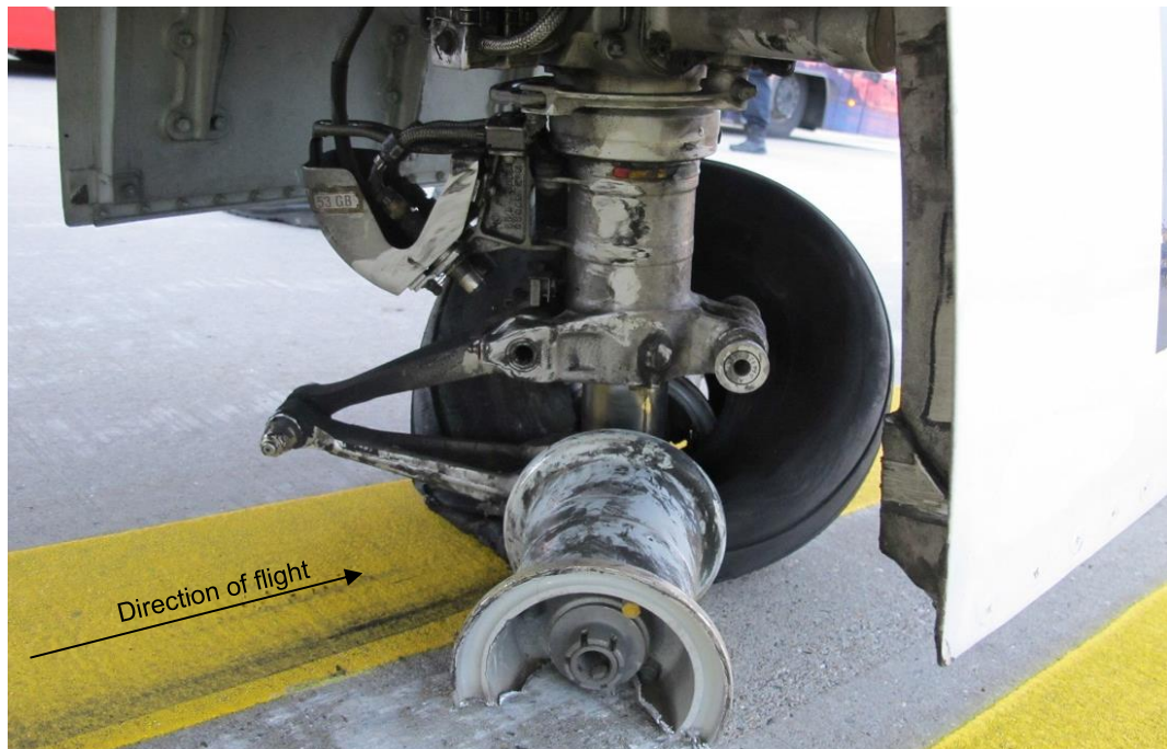
Figure 7: Damage to the nose gear of D-ANFE after landing; the left tyre got blocked between wheel rim, landing gear strut and axle.
