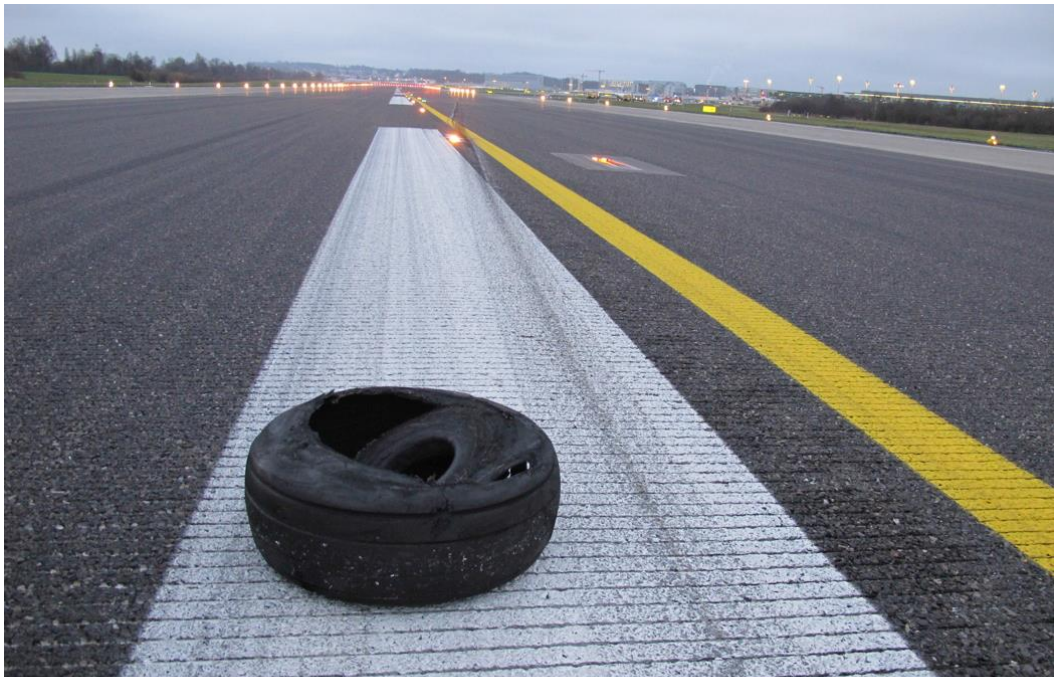
Figure 5: During the inspection of runway 14 after the landing of D-ANFE the tyre of the right nose wheel was found approximately 2080 m from the runway threshold. Beside it, white and black traces are visible.
