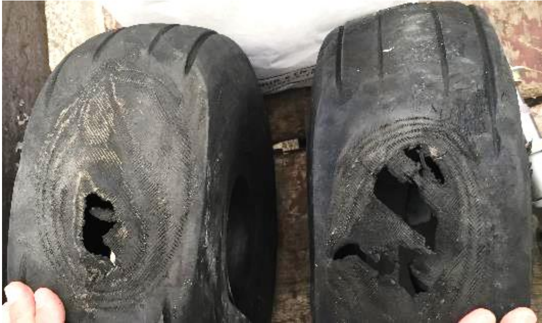
Figure 8: Abrasion mark on each of both nose wheel tyres of D-ANFE
