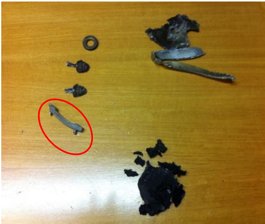
Figure 9: Small parts of the nose gear found on runway 14
