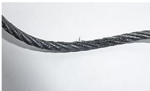
Illustration 6: Damaged control cable where in contact with the front top-left pulley
