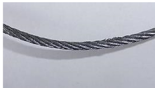
Illustration 7: Damaged control cable where in contact with the front top-right pulley
