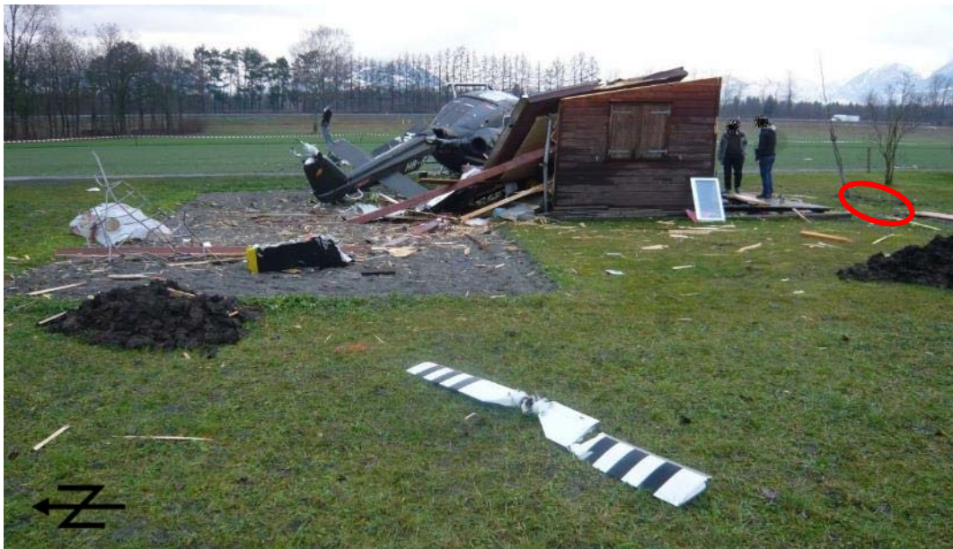
Illustration 10: Final position of the wreckage and tail rotor with crosshead lying underneath. The tail rotor was located on the ground – viewed in the approach direction – approximately 10 metres in front of the helicopter's impact point (circled in red).
