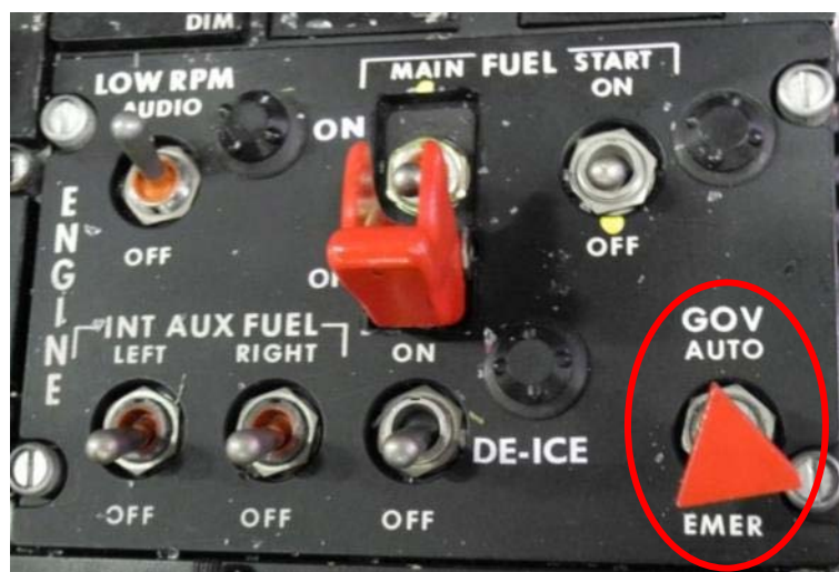
Illustration 8: Engine control panel with governor switch (circled red).
