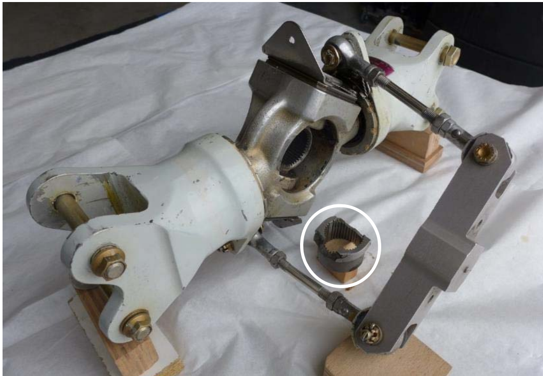
Illustration 19: Tail rotor hub with pitch links, crosshead and static stop (circled white) with broken-off flanges
