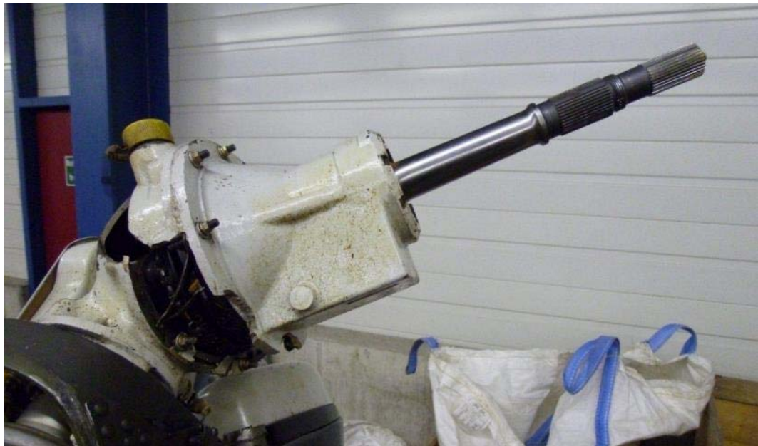
Illustration 12: Burst-open housing of the tail rotor transmission. The fact that the tail rotor driveshaft appears to be intact is remarkable.
