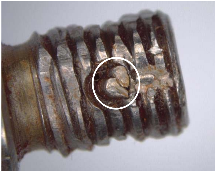
Illustration 22: End of the pitch change rod with sheared-off thread and split pin (circled white).
