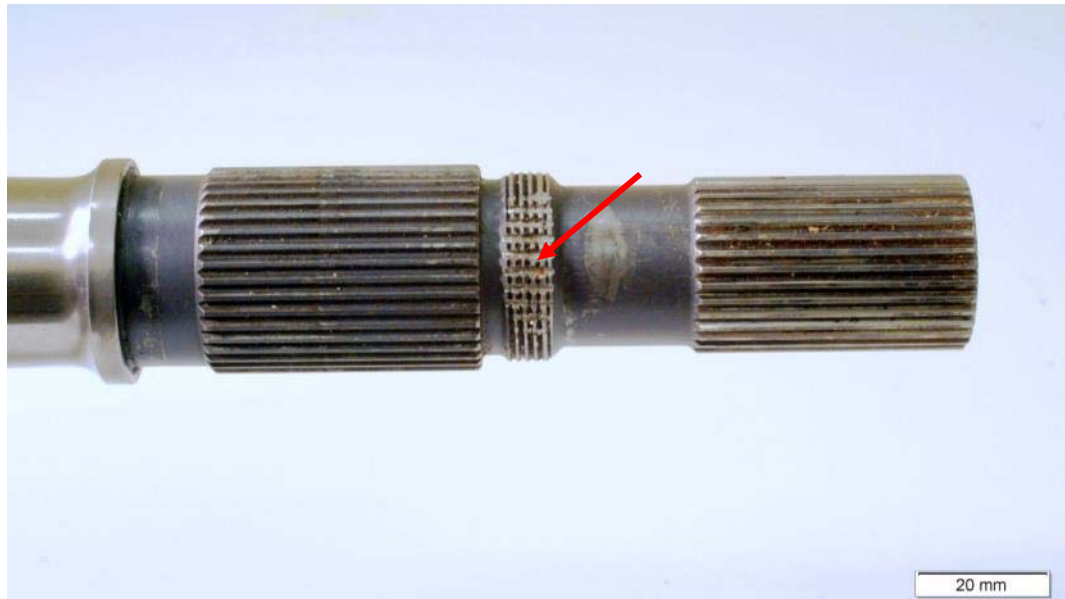
Illustration 18: Tail rotor driveshaft with visible notches on the thread for fitting the retaining nut (red arrow)
