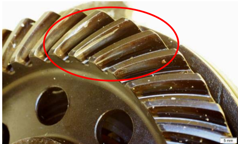
Illustration 16: Damaged tooth flanks of the bevel gear (circled red)
