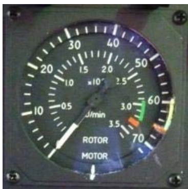
Illustration 3: The cockpit instrument displays the rotor speed in the inner circle and the engine (power turbine) speed in the outer circle.
