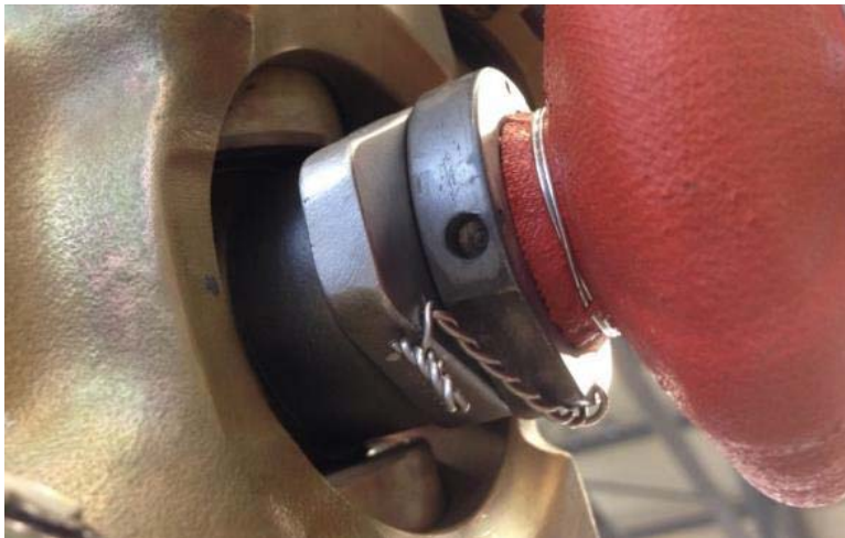
Illustration 5: Tail rotor hub with static stop and wire-locked retaining nut (picture of tail rotor system of same type).
