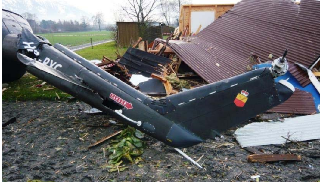
Illustration 11: Burst-open tail rotor transmission with tail rotor driveshaft.
