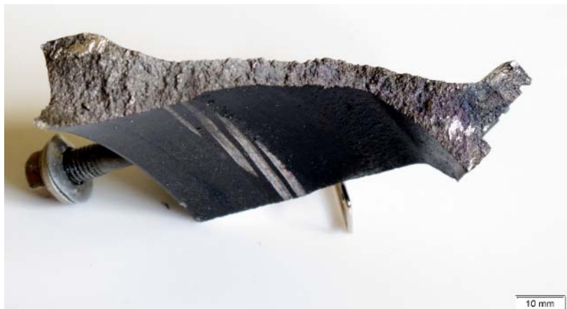
Illustration 14: Burst segment with helical marks
