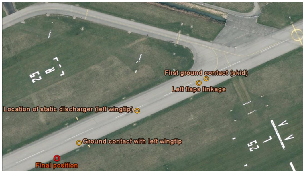
Figure 4: Final position of HB PLC (red) and distinctive features as a result of the landing of HB-PLC on runway 25.
