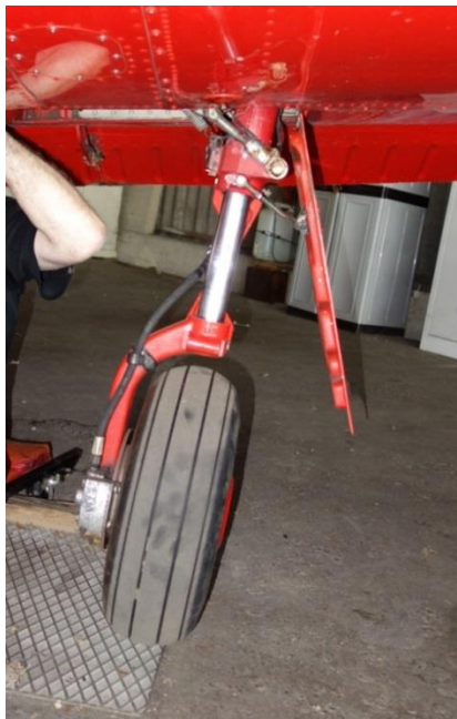
Figure 7: Left main landing gear of jacked-up HB-PLC in its incompletely extended position
