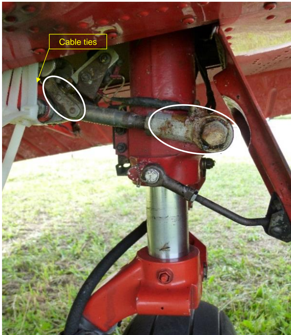
Figure 6: Left main landing gear of HB-PLC with cable ties (yellow arrow) and clear grease marks on the outside of the landing gear link (white frame)
