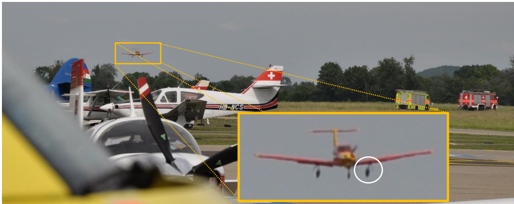
Figure 1: HB-PLC on final approach to runway 25 (hard surface) at Grenchen regional airport (LSZG) with incompletely extended landing gear (white circle).
