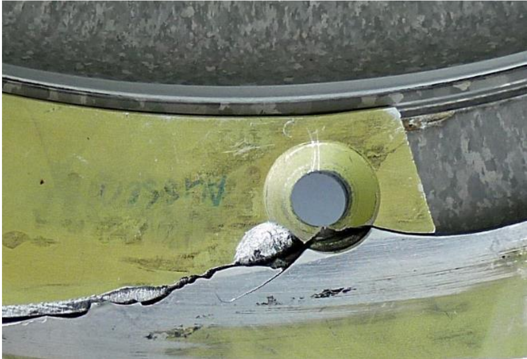
Illustration 14: Deep impact wear in the countersink and distinct abrasion marks on the broken-off segment.
