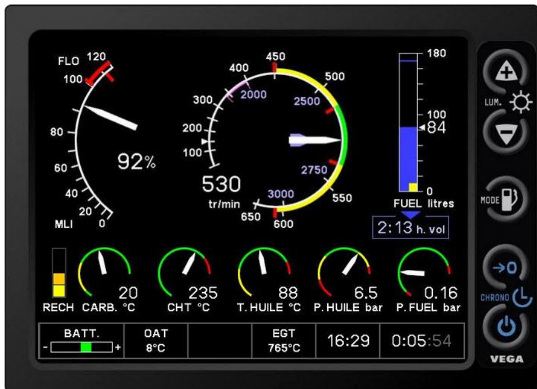
Illustration 5: Image of the EPM with French labels and SI units.
