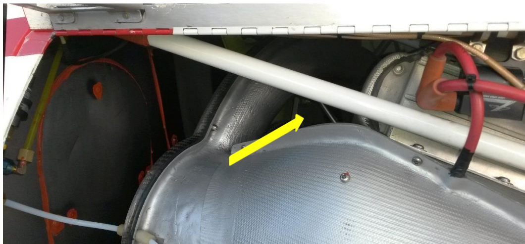
Illustration 3: View of the air cooling system in the engine bay. The yellow arrow points to the area of the air intake.
