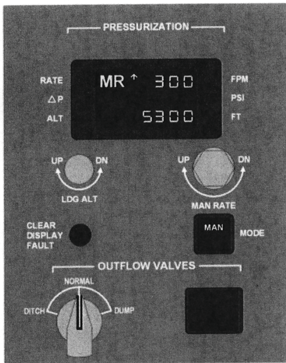
Cabin Altitude for Aircraft Cruise Altitude in Manual Mode
