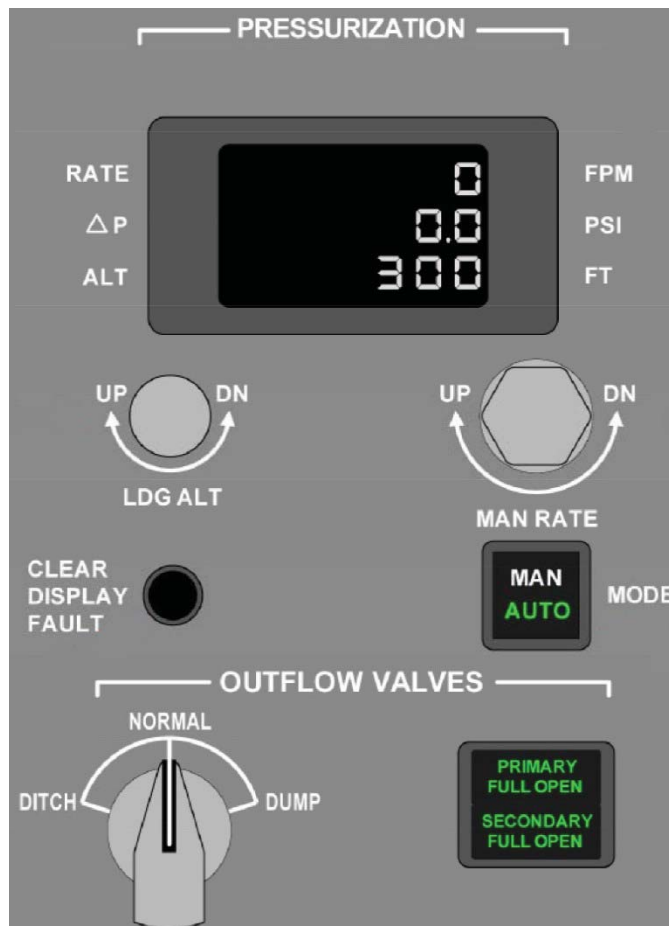
Figure 2: Cabin pressure controller (CPC)
