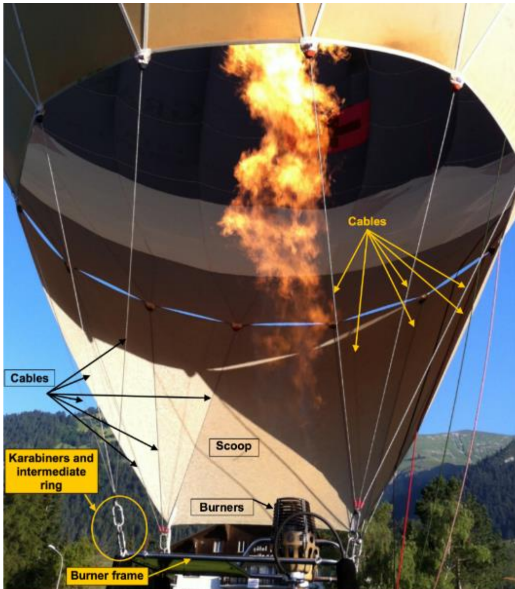
Figure 10: Photograph taken before the take-off of the accident flight, showing the scoop, the burners and the cables of the envelope connected to the burner frame.
