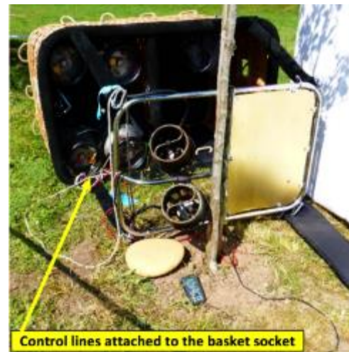
Figure 4: Final position of the basket with the burner frame.
