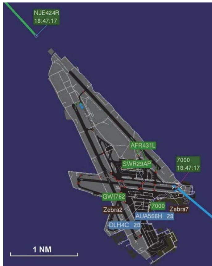
Illustration 2: Recording of the ground radar SAMAX with highlighted flight paths of NJE 424R (green) and HB-PLY (blue) at 18:47:17 UTC, shortly before the go-around of HB-PLY.
