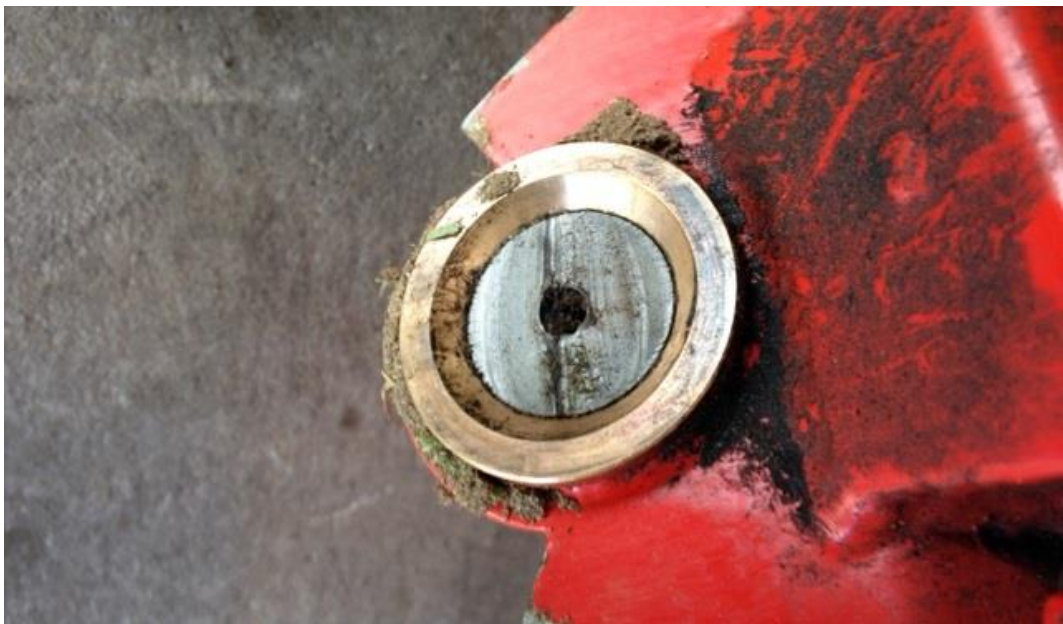
Figure 13: Fractured steering axle of D-EGPZ
