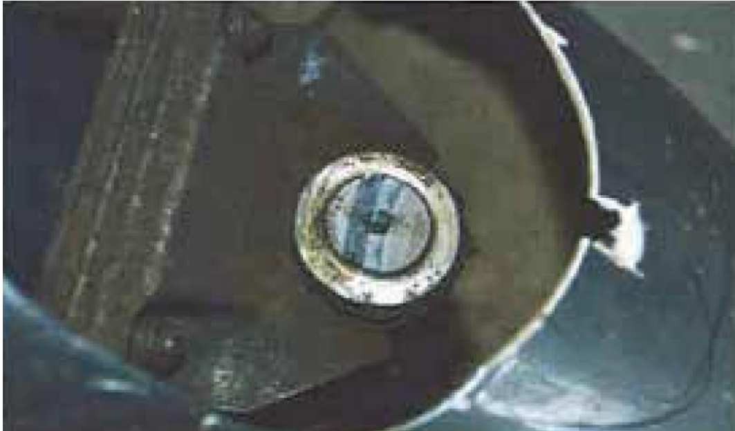
Figure 12: Fractured steering axle of G-EMSA (AAIB Bulletin 11/2014)
