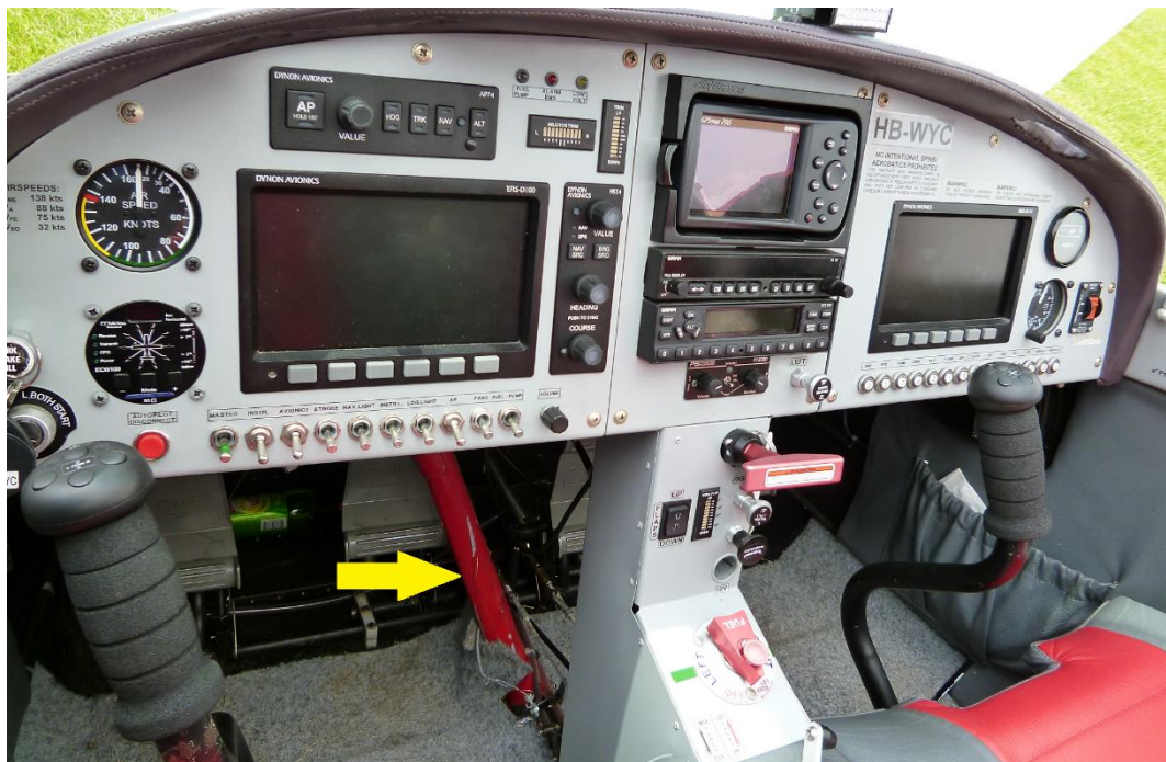
Figure 4: Cockpit of HB-WYC; the yellow arrow indicates the broken-off leg of the nose landing gear which penetrated the cockpit
