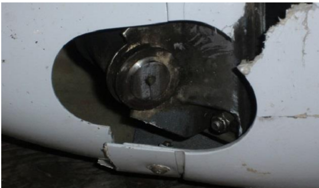
Figure 14: Fractured steering axle of D-EMNA
