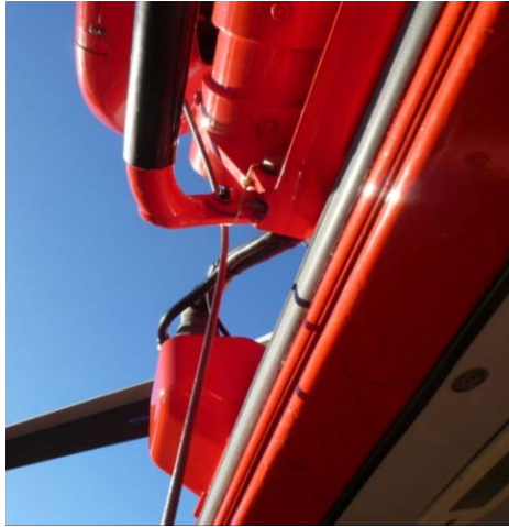
Figure 12: The visible range for the hoist operator if he leans out of the cabin and looks upwards, as illustrated in Figures 10 and 11.
