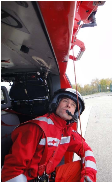
Figure 10: Required working position of the hoist operator to identify a possibly snagged hoist cable.
