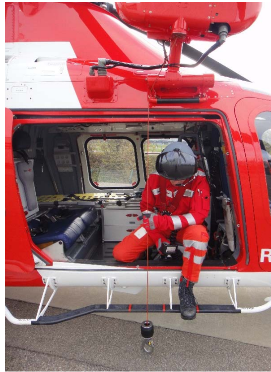
Figure 7: Hoist operator's working position in the case of a snagged cable. The lateral cable offset is approximately 15 cm compared to the normal cable position.
