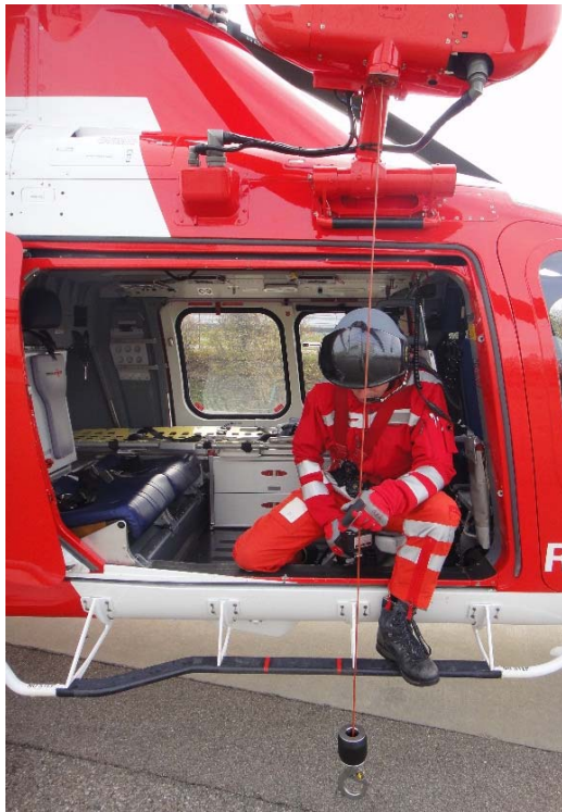
Figure 6: Hoist operator's working position in the case of a normal cable position. The red markings on the step show the limits for the longitudinal position of the hoist cable. They were added after an incident not related with this case based on an airworthiness directive (AD).
