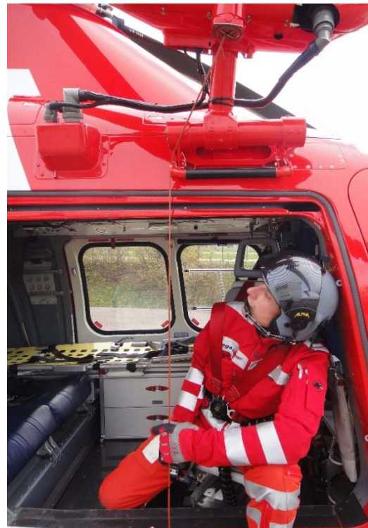
Figure 11: The hoist operator must lean forward until he is below the upper door frame in order to be able to see the rescue hoist.
