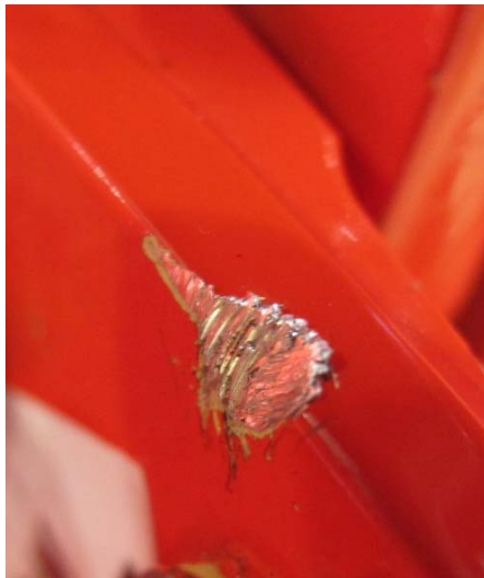
Figure 4: Detail of the damaged edge of the flat bracket with the imprint of the surface structure of the cable.
