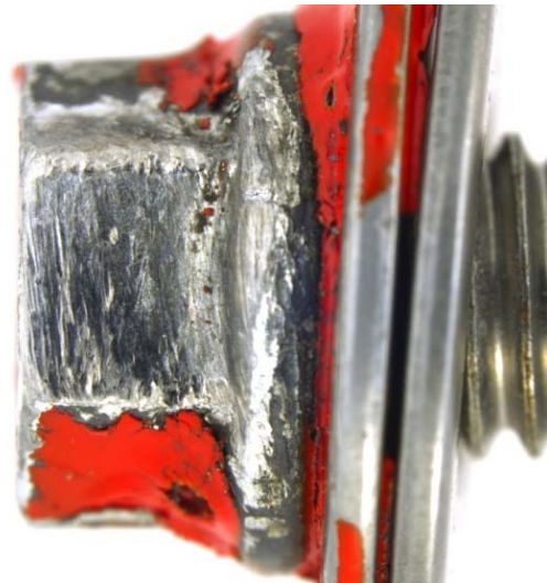
Figure 5: Detail of the damaged nut (Item 29) and washer (Item 28).
