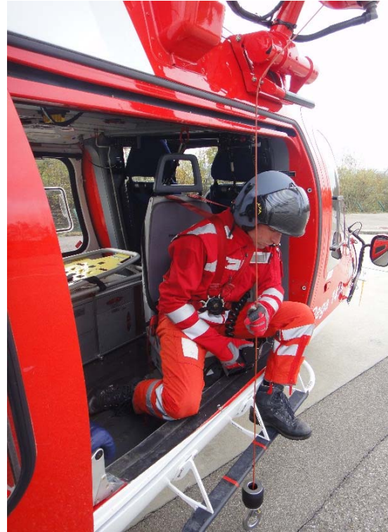
Figure 9: Hoist operator's working position in the case of a snagged cable. The cable hangs closer to the step bar compared to the normal cable position.
