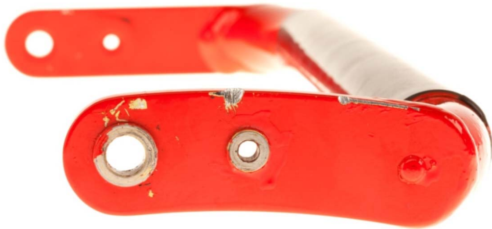
Figure 3: Handle assembly with the damaged flat bracket (for detail, see Figure 4).
