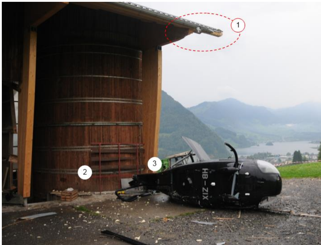
Figure 3: Final position of the wreckage: ① Point of collision ② and ③ location of the passengers at the time of the accident.
