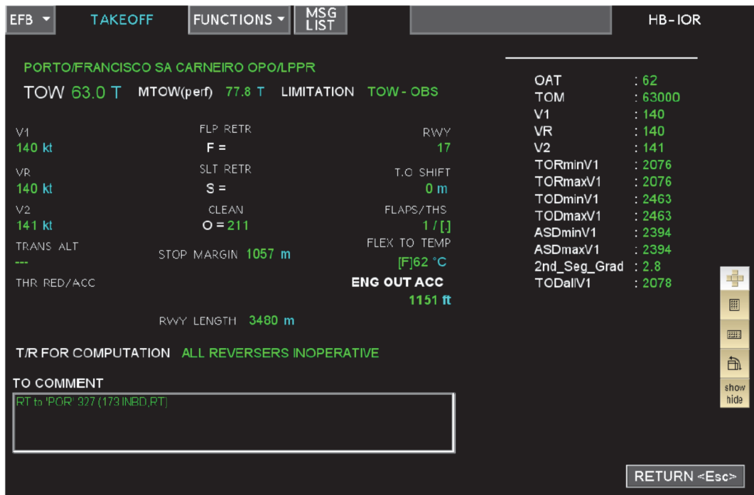
Figure 2: Results of the takeoff performance calculation on the screen of an EFB
