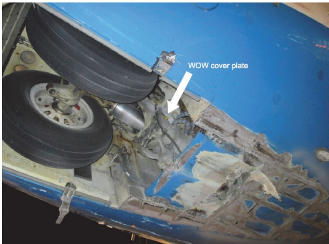
Figure 7: The nose landing gear WOW cover plate trapped between the upper and lower drag struts of the nose landing gear. This photo was taken at the scene of the accident.
