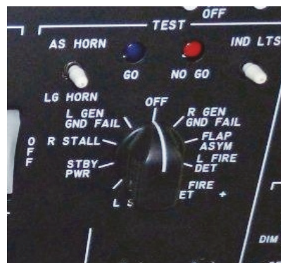
Figure 1: Master test switch
