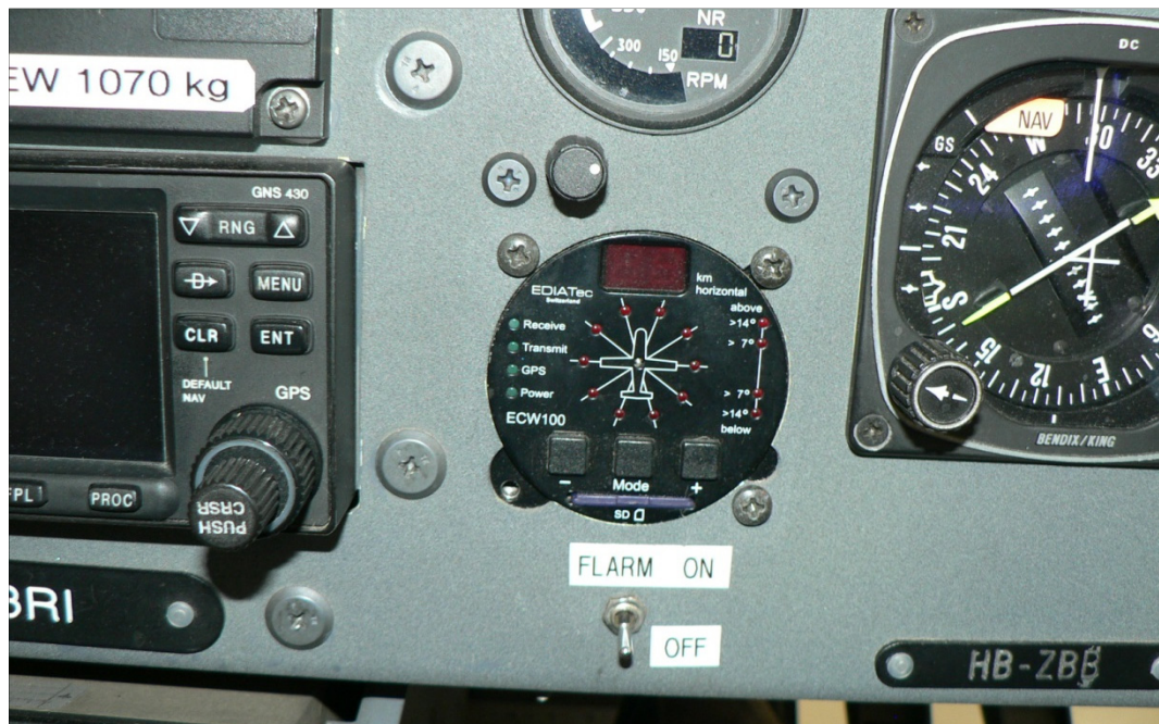
Figure 6: Ediatec ECW100 FLARM on the instrument panel of HB-ZBB. The relative position of other aircraft is displayed in the horizontal plane by the circle of LEDs in the middle of the display; in the vertical plane it is displayed by the LEDs on the right edge. The upper digital display gives the horizontal distance in 100 m increments (e.g. 0.1 km).
