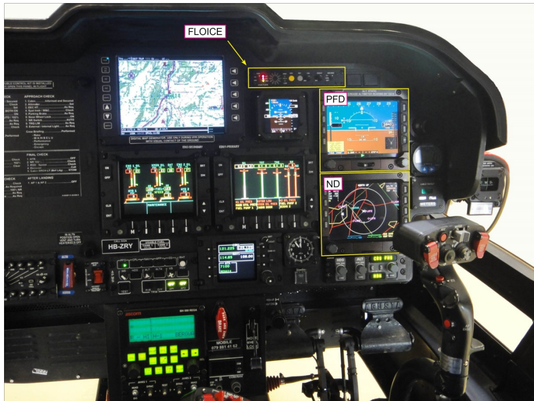
Figure 9: HB-ZRY instrument panel (Photo: Rega). The PFD and ND are on the right. The FLOICE is to the left above the PFD.
