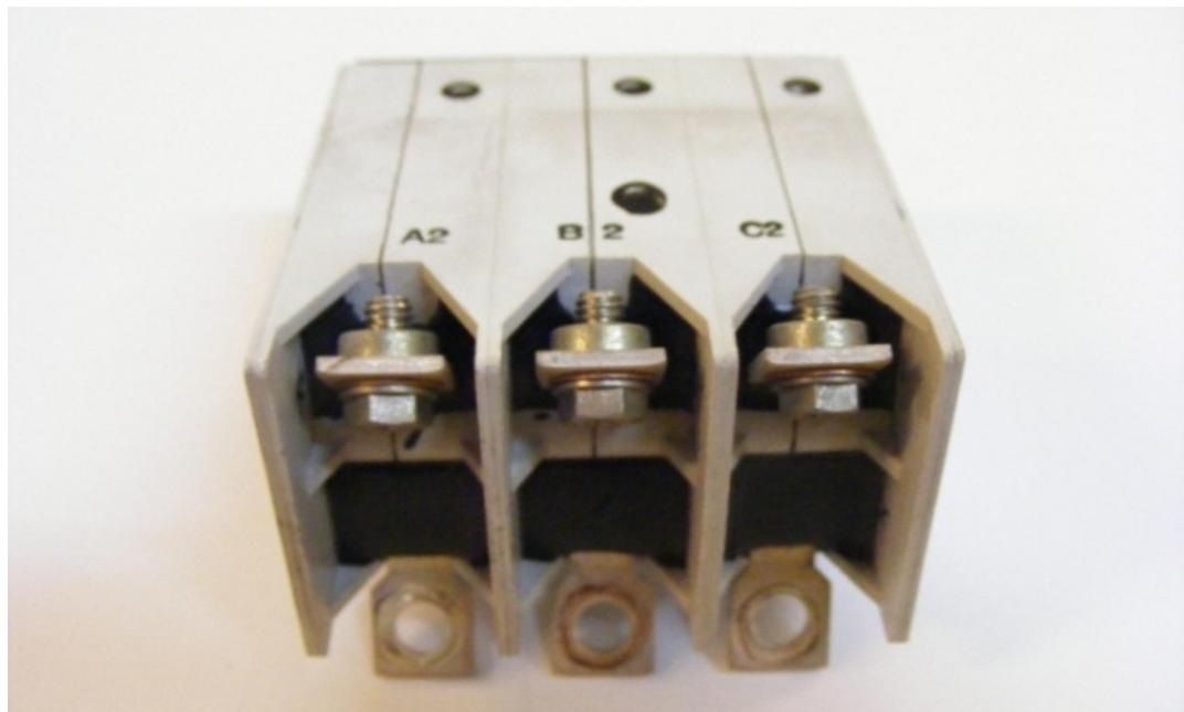
Figure 5: Circuit breaker 3XN1 before the test (source: Airbus)
