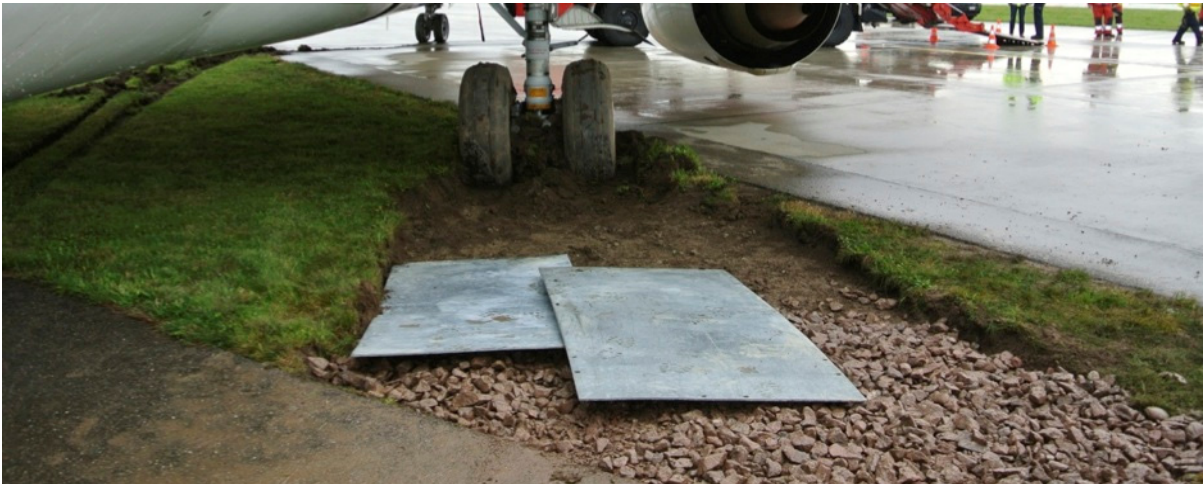
Figure 21: Removal of the earth behind the right main landing gear, creation of a weight-bearing base, right: de-icing lane F2
