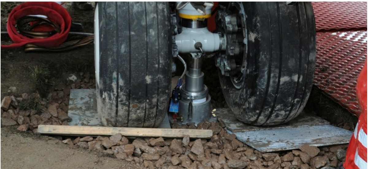
Figure 22: Right main landing gear. Jacking of the landing gear and insertion of a hard base
