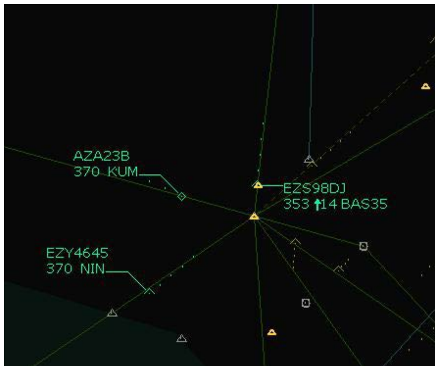
Fig. 5 First appearance of the radar label of flight EZS 98DJ on the screens of sector L56
