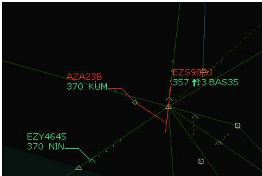
Fig 6 The STCA is triggered in Geneva sectors L34 and L56
