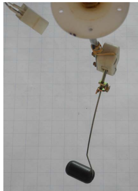
Figure 10: Float in skewed position
