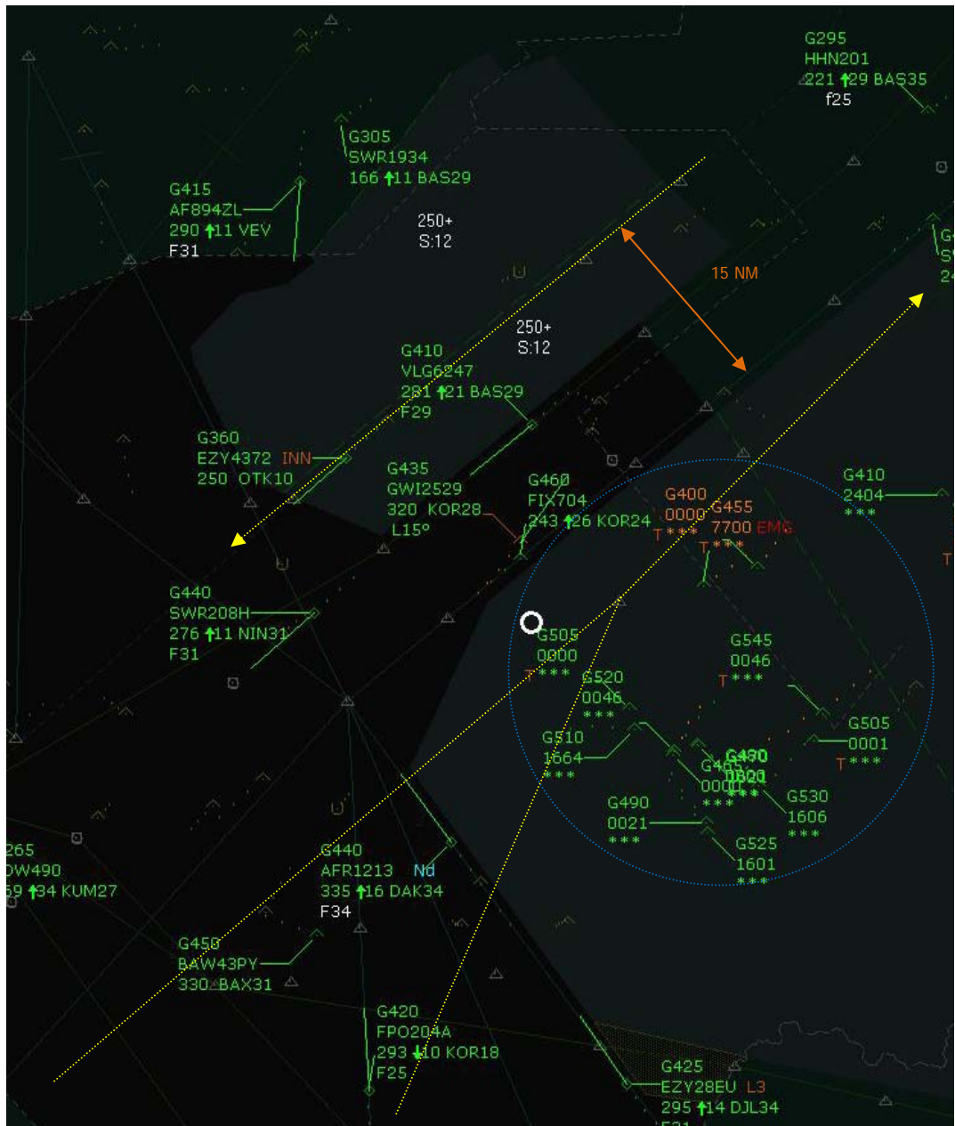
Figure 5: Radar image of Sector L12 in Geneva ACC at the time of the first radio contact with GWI 2529 at 08:33:40 UTC. The blue circle shows the area in which additional transponder codes or symbols of aircraft are shown which are normally suppressed.
