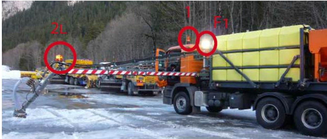
Figure 2: Airport de-icer with warning lamps 2L and F1 (photo does not date from the day of the accident).
