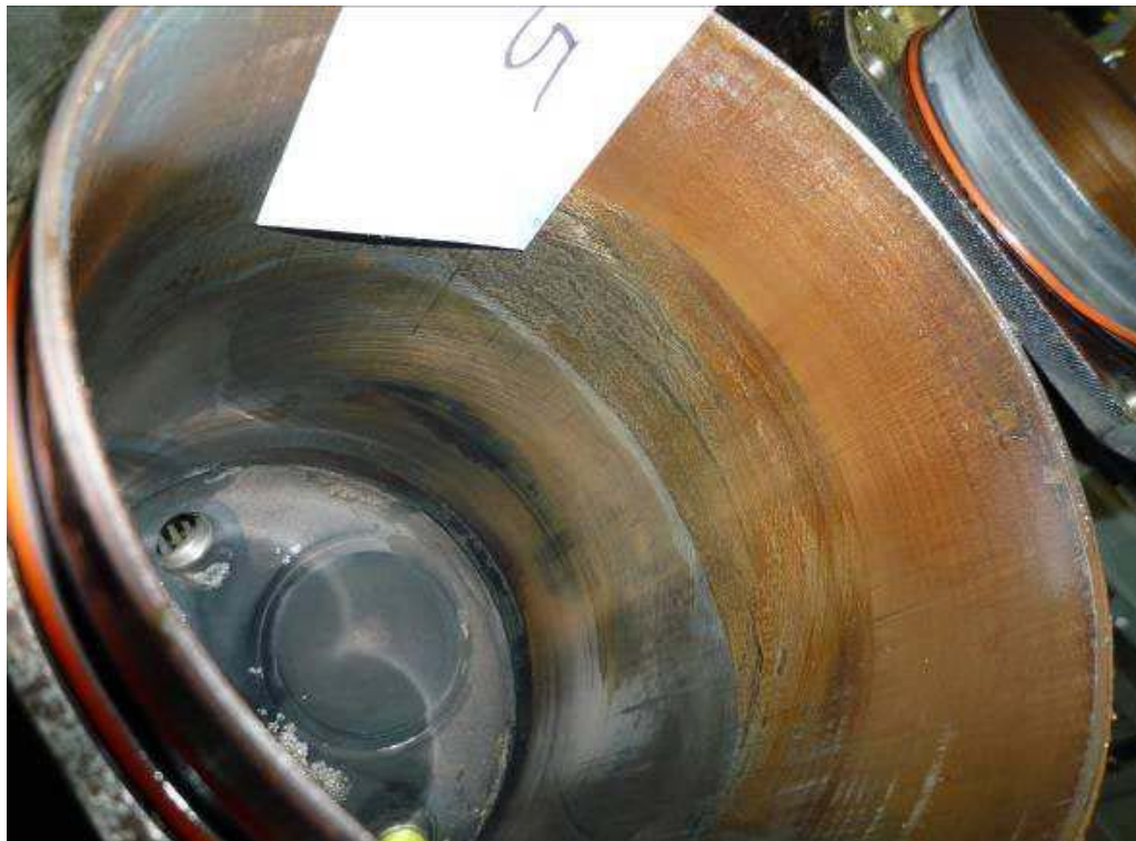
Figure 3: Cylinders 5 and 6 exhibit pronounced corrosion on the cylinder wall
