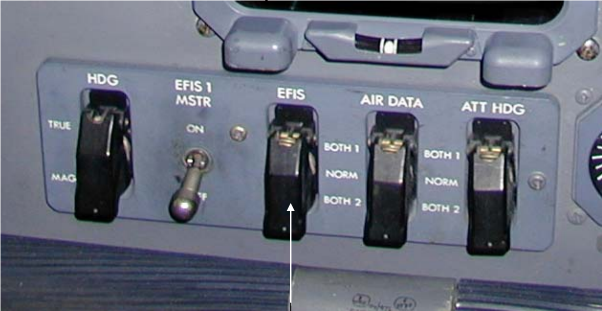
Switch for EFIS displays In "BOTH 2" position, for example, the data from PFD2 / ND2 are copied to PFD1 / ND1.
