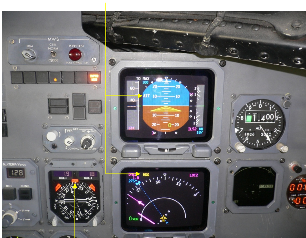
DBI (distance bearing indicator) with red heading flag
