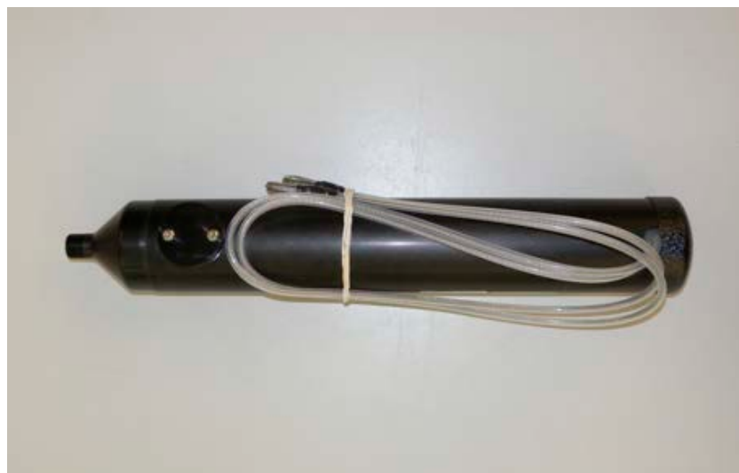
Fig. 11: Rocket motor with release/igniter unit
