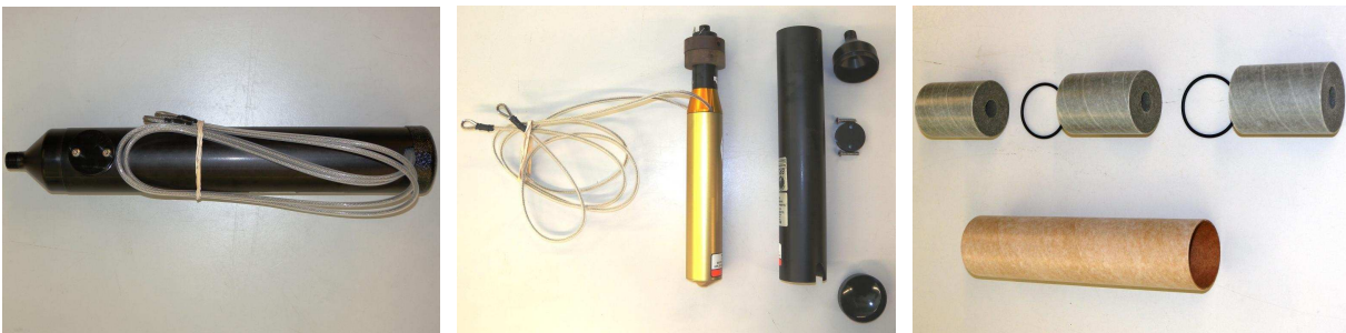
Fig. 1: Main components of the BRS 440 rocket; the 3 gray cylinders at the top of the rightmost picture compose the rocket motor.
