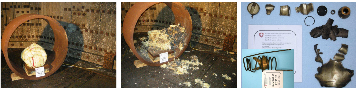
Fig. 10: SCO of the BRS 440 rocket; respectively before and after test and the fragments.
