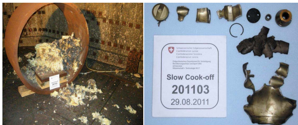
Fig. 12: Test results and fragments
