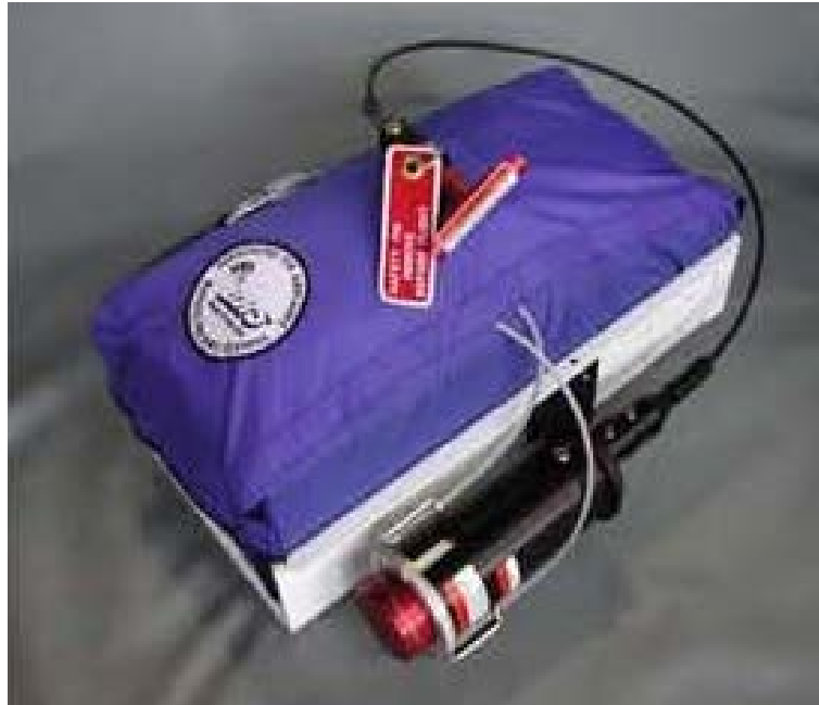
Fig. 8: Parachute packed in bag with Velcro seal
