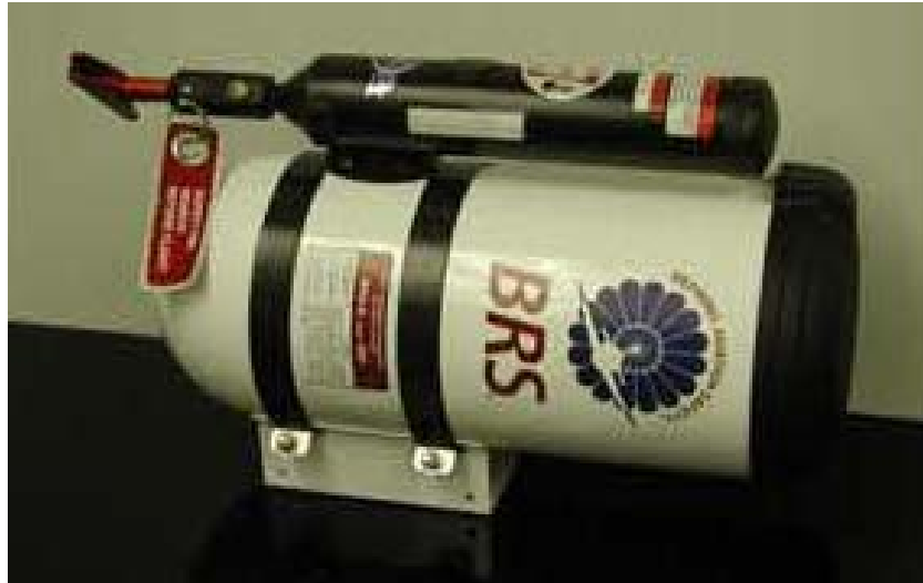
Fig. 6: Parachute packed in canister
