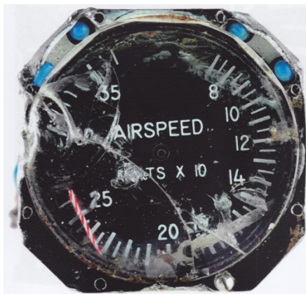
Figure 4: standby airspeed indicator
