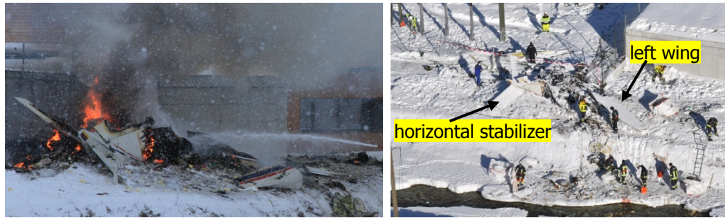
Figures 2 und 3: Horizontal stabilizer and tailcone (left); Debris after extinguishing the fire (right)
