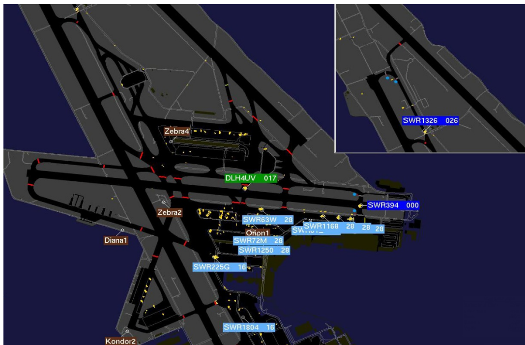
Figure 11: SAMAX ground radar screen. The northern part of the runway system is shown in a separate box (inset) on the screen.
