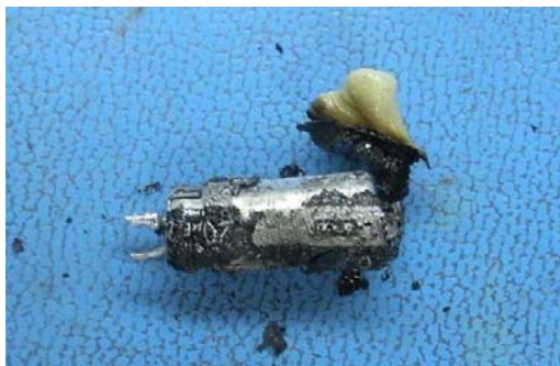
Fig. 6: Condensateur C12 surchauffé
