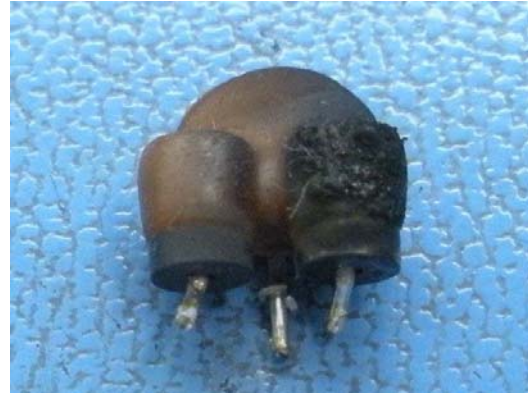
Fig. 9: Damaged inductor FL2
