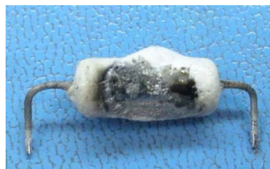
Fig. 7: Capacitor R7 damaged
