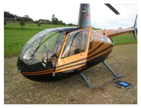
Annex 1: Final position of the helicopter with embedded landing skids
